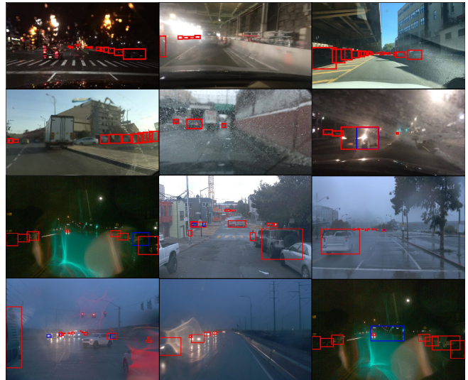
Fig. 5: Example of performance drop encountered by the object detection system. Red and Blue coloured boxes represent the false negative and false positive error made by the object detector in each input frame. 1 st and 2 nd rows represent Faster RCNN and RetinaNet detection performance for primary dataset KITTI and secondary dataset BDD. 3 rd and 4 th rows show Faster RCNN and RetinaNet performance for primary dataset BDD and secondary dataset Waymo. In all cases, the mAP is lower than 0.4, and detection confidence is higher than 0.5.
