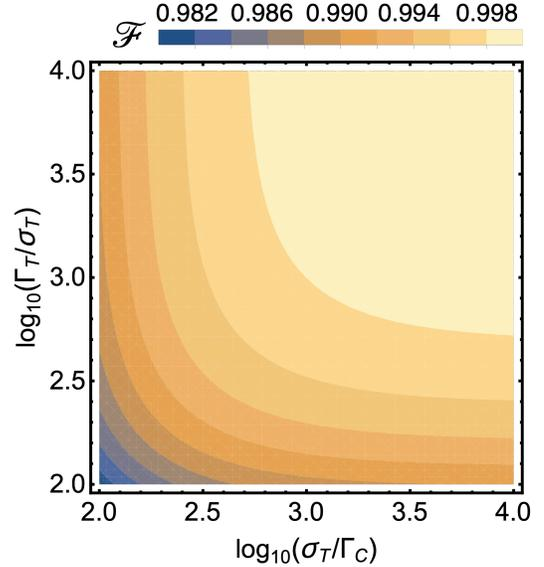
FIG. 2. Gate performance. Contour plot of the fidelity  $\mathcal{F}$  versus  $\Gamma_T/\sigma_T$  and  $\sigma_T/\Gamma_C$  for  $\Delta_T = 0$  and Lorentzian lineshape for the input single-photon pulse of the target qubit.
