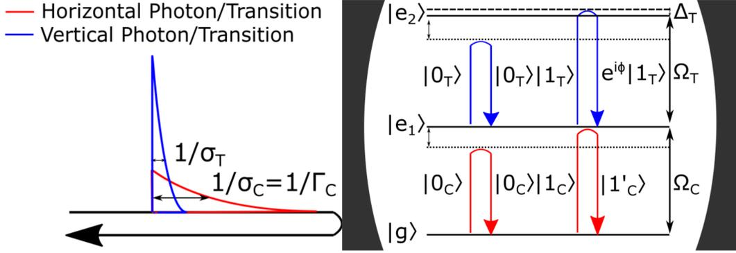
FIG. 1. Gate schematic. The control photon and the control transition  $|g\rangle \leftrightarrow |e_1\rangle$  of the ladder system are horizontally polarized, and the target photon and target transition  $|e_1\rangle \leftrightarrow |e_2\rangle$  are vertically polarized. The detuning  $\Delta_T$  of the central frequency of  $|1_T\rangle$  relative to  $\Omega_T$  controls the controlled-phase  $\phi$  imparted on the target photon.
