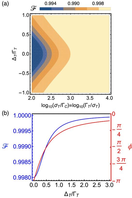
FIG. 3. Tunability of the controlled-phase gate. **(a)** Fidelity  $\mathcal{F}$  versus detuning  $\Delta_T$  and  $\sigma_T/\Gamma_C = \Gamma_T/\sigma_T$ . **(b)** Phase  $\phi$  in radians and fidelity  $\mathcal{F}$  versus the detuning  $\Delta_T$  when  $\sigma_T/\Gamma_C = \Gamma_T/\sigma_T = 10^3$ . Note that the conditional phase starts near  $-\pi$  and goes to zero from the negative side, indicating a phase lag.
