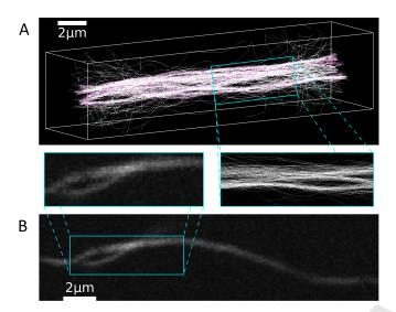
**Fig. 4.** Hole defect observed in simulation and experiment. (A) Simulation of a big bundle with 225 filaments (white) and approximately 16000 cross links (pink). (B) Fluorescent confocal laser scanning image of a collagen bundle. Those parts of both images showing the hole defect are magnified and compared side-by-side in the center panel of this figure.
