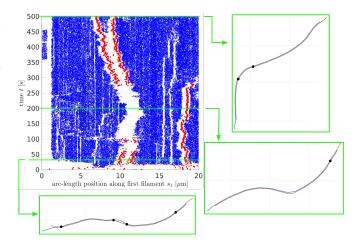
**Fig. 3.** Dynamics and interactions of defects observed in numerical simulation. The position of braids (red dots) and cross links (blue dots) along the (first, i.e., blue) filament is tracked over time. The inset images (green frames) show the corresponding configuration of the two filaments (blue and red lines) and the braids (black dots) in the bundle at three different time points.
