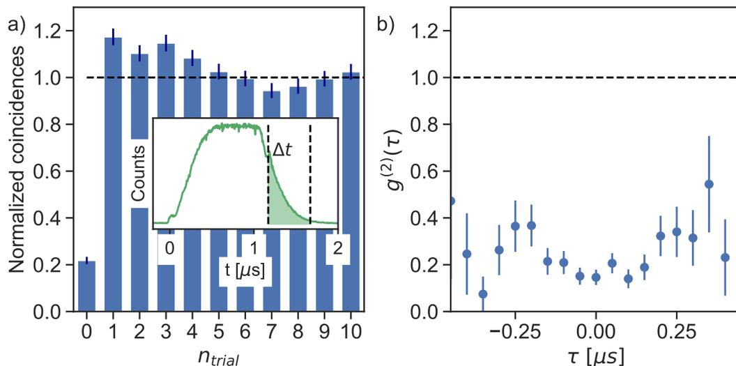
Figure 10: Single-photon generation: example of single-photon generation with  $\Delta t = 500$  ns. (a) Normalized coincidence counts between different trials, leading to a value of  $g_{\Delta t}^{(2)} = 0.218 \pm 0.015$  for  $n_{trial} = 0$ . (b) Time-resolved measurement of  $g^{(2)}(\tau)$  leading to a zero-delay value of  $g^{(2)}(0) = 0.15 \pm 0.03$ . Error bars correspond to one standard deviation.
