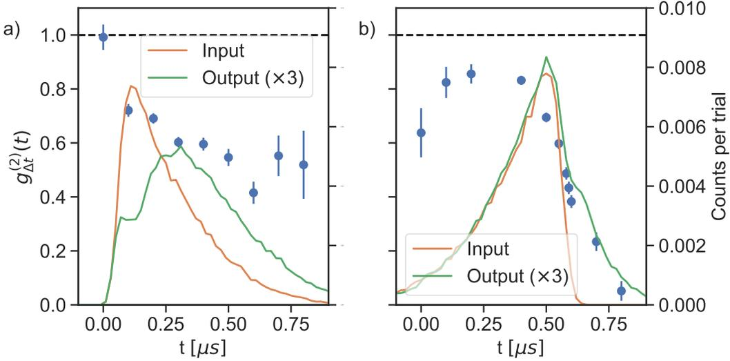
Figure 4: Transients for triangular pulses. Second-order autocorrelation function (in blue) for a window  $\Delta t$  of 200 ns along the output pulse, temporal distribution of the input (in orange) and output (in green) pulses for an input pulse with a pseudo-triangular shape and a negative slope (a) and for an input pulse with a positive slope (b). The error bars correspond to one standard deviation.
