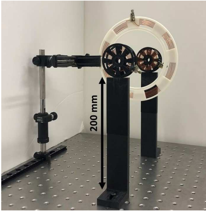
Fig. 5: A rotated view of the experimental setup showing (from foreground to background) a given instance of the TX, IC, and RX variations.
