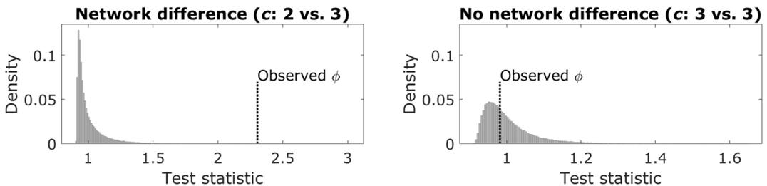
FIG. 10. The empirical distribution of the ratio statistic  $\phi_{\mathcal{L}}$  is generated by the permutation on two groups each consisting of ten modular networks. Here, we test if there is group difference in networks with parameters  $c = 2$  vs. 3 (left) and 3 vs. 3 (right). As expected, the test based on the topological loss rejects the null hypothesis when there is group difference (left) while it does not reject when there is no difference (right).
