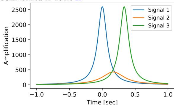
FIG. 10: Signals generated for a triangular configuration. Each signal corresponds to each station detecting the axion flux due to a nearby AQN. From these signals we can obtain the parameters  $t_i$  and  $\tau_i$  in order to solve the system of Eqs. (12)
