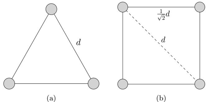
FIG. 5: Two network configurations for the detection of axions: (a) An equilateral triangle, and (b) a square network. Optimally, stations (grey circle) are separated by a distance  $d \simeq 100$  km. 94% (resp. 100%) of the trajectories are uniquely determined in a triangular (resp. square) network. A triangular network has the highest event rate per station.
