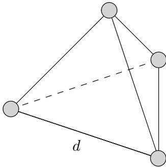
FIG. 6: A base unit of the X-ray array of detectors. It consists of four detectors (grey circles) located at the vertices of a regular tetrahedron, separated by  $d = 50$  m.
