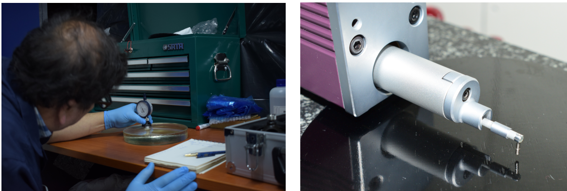
Figure 4. Left: Sphericity measurement of the mandrel. If sag measurements are constant within 1 \mu m over the whole surface the mandrel is considered acceptable. Right: CFRP replica surface profiling. Profiles must be perpendicular to the fibers orientation of the first CFRP layer.
