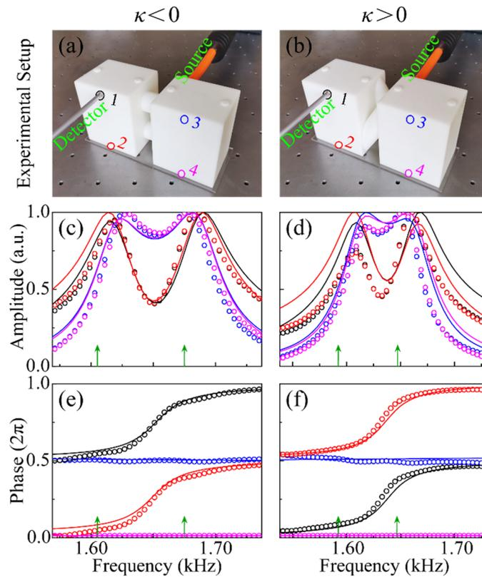
FIG. 2. (a) and (b): Experimental setups for testing the hopping signs of the straight-linked and cross-linked double cavity systems, respectively. The acoustic
