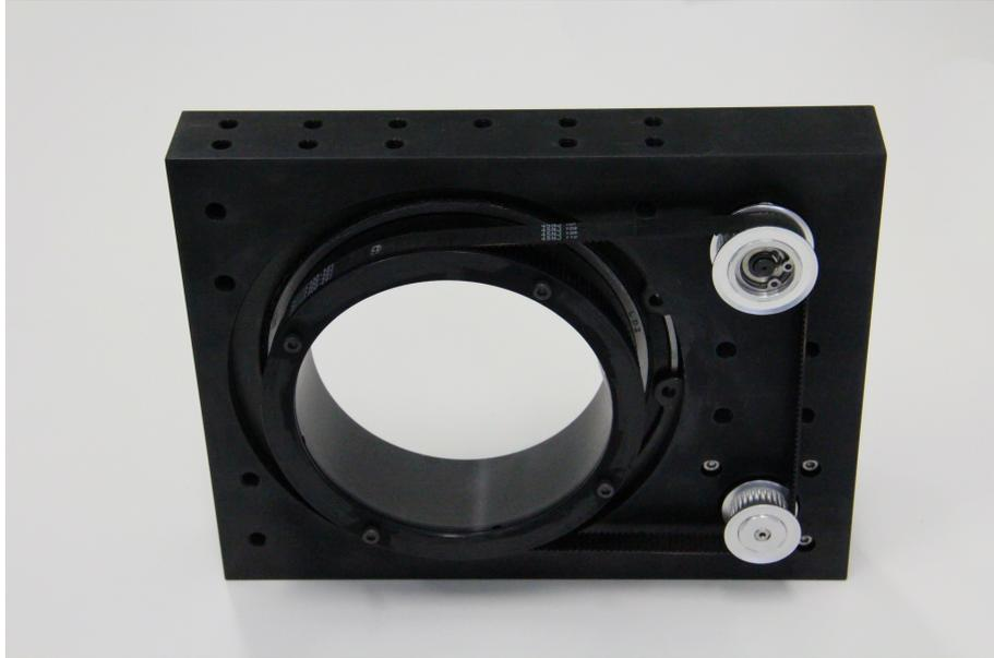
Figure 2. Phase screen in its rotating opto-mechanical mount as delivered by SILIOS. The screen is designed to work in transmission. Rotation is performed using a stepper motor controlled over USB using a dedicated software.
