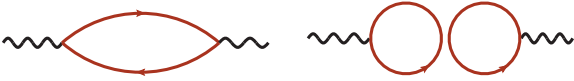
Fig. 2. The quark-connected (left) and quark-disconnected (right) Wick contractions for the LO-HVP in the isospin limit.
