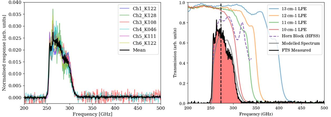
Figure 14. (Left) The FTS measured optical response of six detectors, one from each of the MUSCAT readout channels, and their mean. (Right) A comparison of a single measured spectrum with a combination of measured optical filter bandpasses and HFSS simulated detector response. The measured spectrum is normalised to match the area of the modelled spectrum and the shapes are in good agreement.
