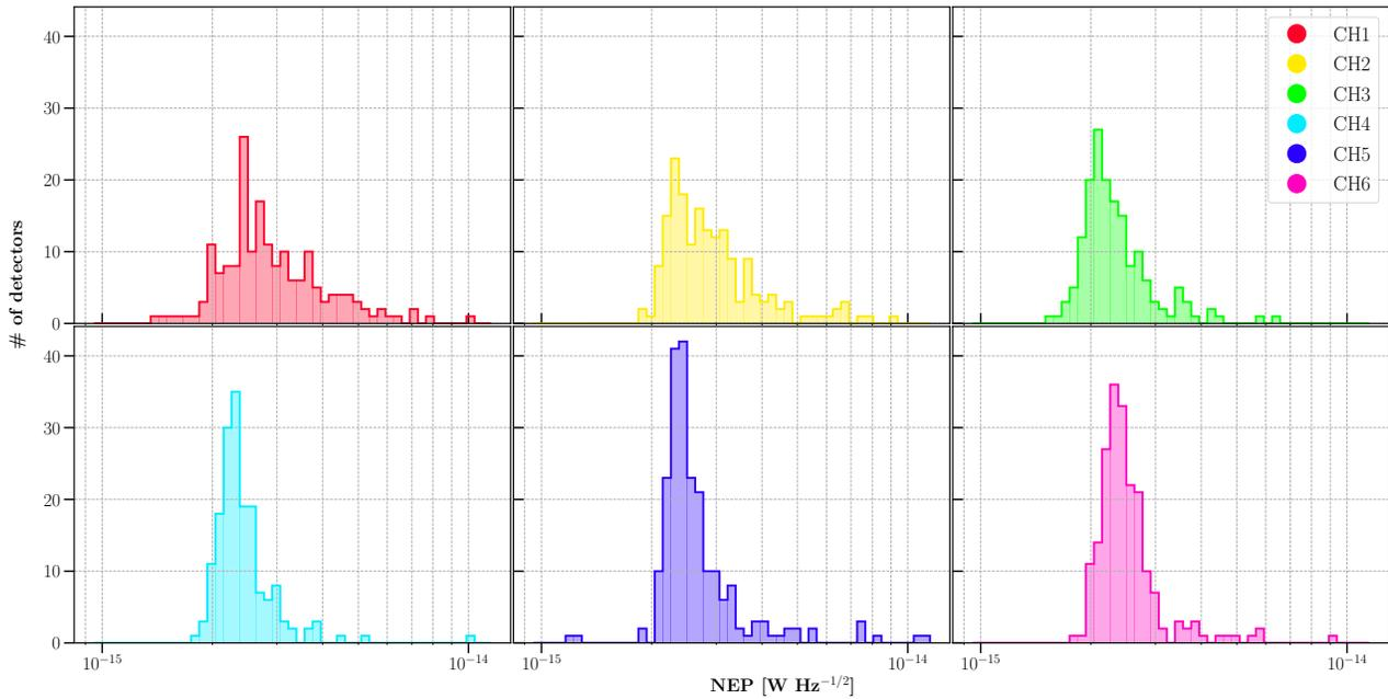
Figure 8. Histograms of the NEP measured under an optical load of  $\sim 300$  K for each of the MUSCAT channels. The maximum accumulation of the distributions at  $\sim 2.4 \times 10^{-15} \text{ W Hz}^{-1/2}$ , very similar to the estimated theoretical noise of  $\sim 2.7 \times 10^{-15} \text{ W Hz}^{-1/2}$ , and the sharp descent of the curves towards less noise, show that the vast majority of the detectors in the MUSCAT focal plane are photon-noise limited.
