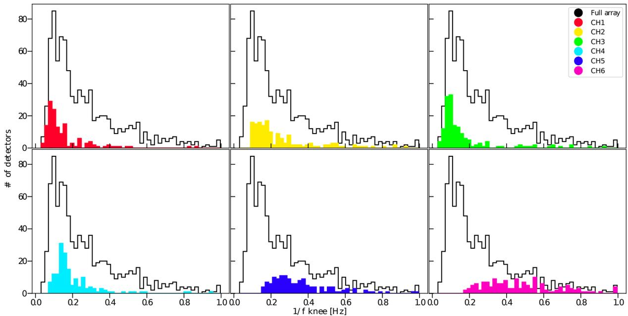
Figure 9. Histograms of the  $1/f$  knee of each MUSCAT channel. The total distribution (solid black line) peaks at 0.1 Hz, although the contributions of each channel move towards a higher frequency reaching maximums from 0.07 Hz (channel 1) to 0.55 Hz (channel 6).
