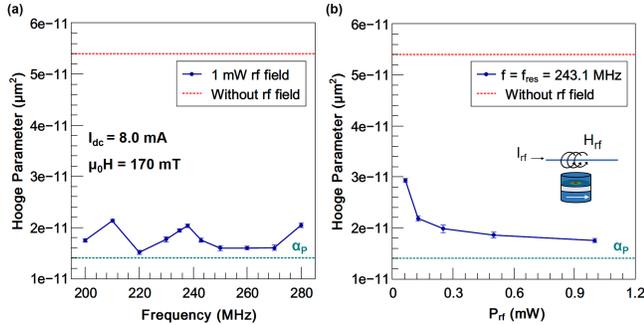
FIG. 3: (a) Hooke parameter in function of the frequency of the applied oscillating field, with fixed  $P_{rf} = 1$  mW. The red line indicates the value measured in the absence of this field. (b) Hooke parameter in function of the power amplitude of the field at a fixed frequency,  $f = f_{res} = 243.1$  MHz. The green dotted lines represent the Hooke parameter measured in the P state.
