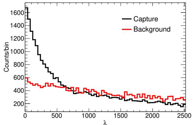
**Fig. 12.** Distribution of the imaging parameter  $\lambda$  for capture and background events for one module of i-TED placed at 50 mm from the sample. Both distributions have been normalized to the integral over the full  $\lambda$  range.
