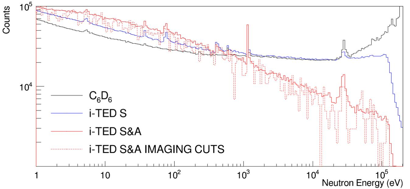
**Fig. 7.** Neutron energy spectra (40 bins per decade) measured with the  $^{56}\text{Fe}$  sample using the i-TED S-detector in singles-mode (blue line) and i-TED with S- and A-detectors in time-coincidence mode (solid red line). The spectrum measured with the  $\text{C}_6\text{D}_6$  detectors is shown in black. The dashed-red spectrum shows the best result obtained with  $\gamma$ -ray imaging cuts. See text for details.
