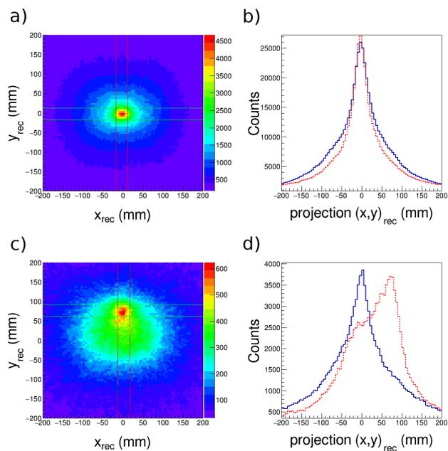
**Fig. 4.** Reconstructed Compton images of a  $^{137}\text{Cs}$  source placed on capture sample position (a), and 10 cm up (c). The lines indicate the projection cuts. b) and d) show the projections of these cuts on both x- and y-axis.
