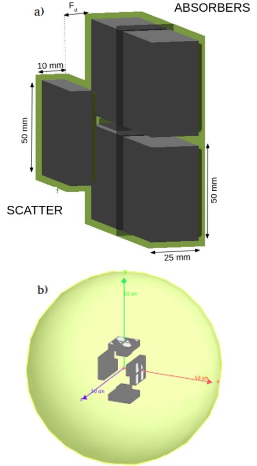
**Fig. 10.** Schematic view of each of the four i-TED modules as implemented in GEANT4 indicating the dimensions of the  $\text{LaCl}_3(\text{Ce})$  crystals of the Scatter and Absorber layers (a). General view of the i-TED detector surrounded by the sphere from which the background  $\gamma$ -rays are emitted (b).
