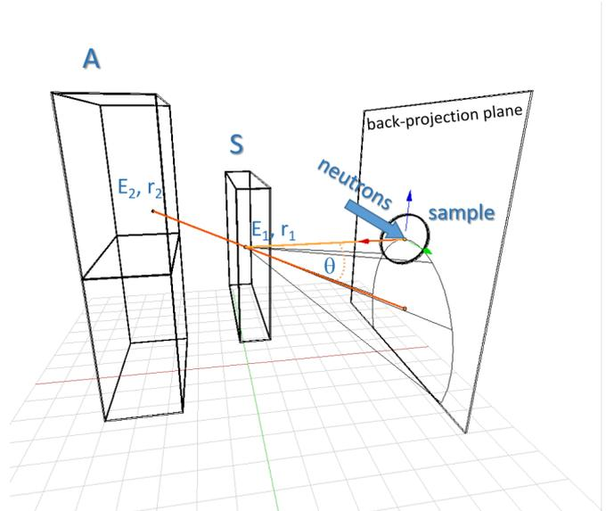
**Fig. 8.** Schematic representation of a capture event validated with i-TED by means of the Compton technique. Measurable quantities ( $E_1$ ,  $E_2$ ,  $r_1$  and  $r_2$ ) correspond to the interaction of the capture  $\gamma$ -ray in both detection layers.
