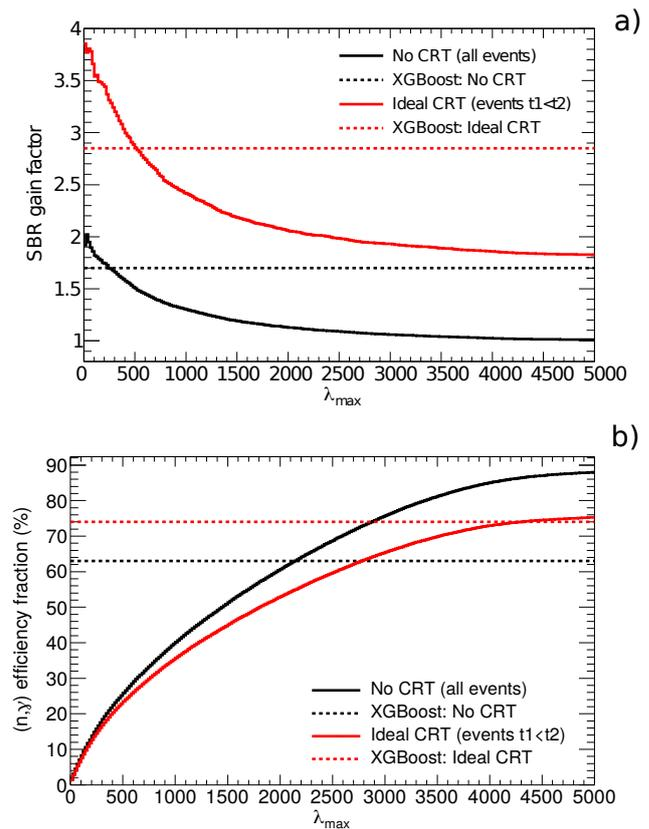
**Fig. 15.** SBR gain factor (a) and fraction of the efficiency for capture events as a function of the  $\lambda$  imaging cut (b). The black and red solid lines correspond to the analytical imaging case with no time resolution and ideal CRT, respectively. The dashed lines show the results obtained with XGBoost.
