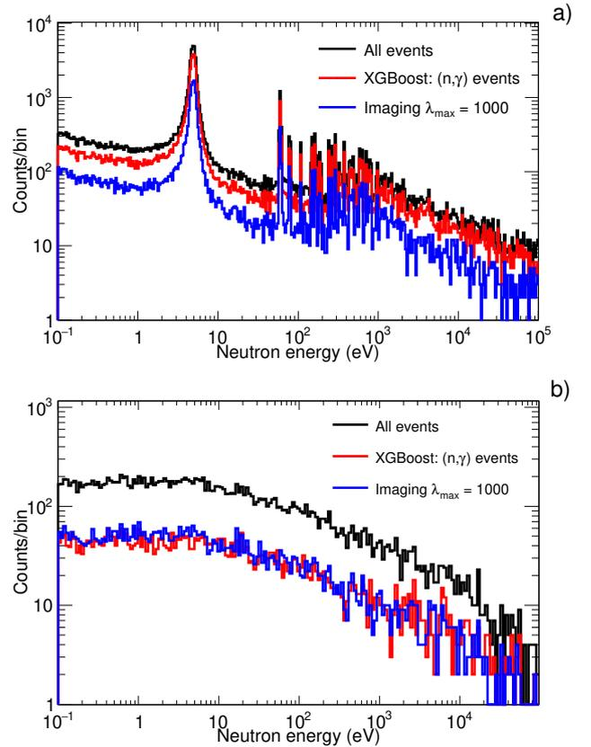
**Fig. 16.** Counting rate as a function of the neutron energy measured with  $^{197}\text{Au}$  (a) and a C-nat (b) samples. The original data set (black) is compared to the fraction of events identified as capture by the XGBoost algorithm (red) and the events selected with an imaging cut  $\lambda_{max}=1000$ .
