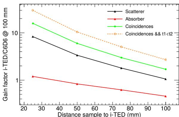
**Fig. 11.** Expected SBR gain factor with respect to a  $C_6D_6$  detector at 10 cm as a function of the i-TED distance to the sample. The scatter (black triangles) and absorber (red triangles) crystals alone are compared to one i-TED module operated in coincidence mode (green solid) and after selection of events with  $t_1 < t_2$  (orange dashed) (see text for details).
