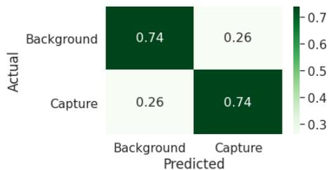
**Fig. 14.** Confusion matrix showing the prediction accuracy of the XGBoost classifier to discriminate capture and background events (see text for details). This result corresponds to the best scenario with ideal CRT.
