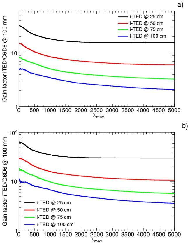
**Fig. 13.** Total SBR gain factor with respect to a  $C_6D_6$  detector at 10 cm as a function of the  $\lambda$  cut. Each curve corresponds to a different distances between the i-TED module and the sample. The two panels correspond to the expected performance of i-TED with no CRT (a) and with an ideal CRT that allows selecting events with  $t_1 < t_2$  (b).
