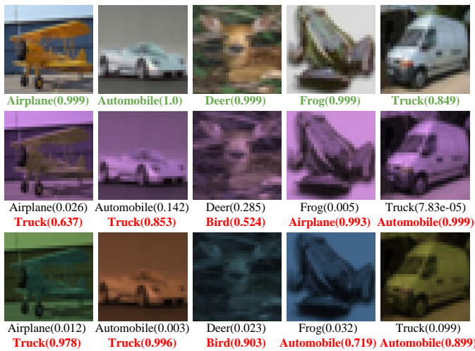
Fig. 5: The sample results depicting the effect of the proposed CCP transformations to fool the CNN using DenseNet model [21]. The 1 st row shows the image classification results over the sample images from the original test set of CIFAR10 dataset [39]. The 2 nd and 3 rd rows present the classification results of the same images after CCP attack with fixed and variable random weight settings, respectively. The class labels with probability for correct and misclassified classes are also shown. Best viewed in color.
