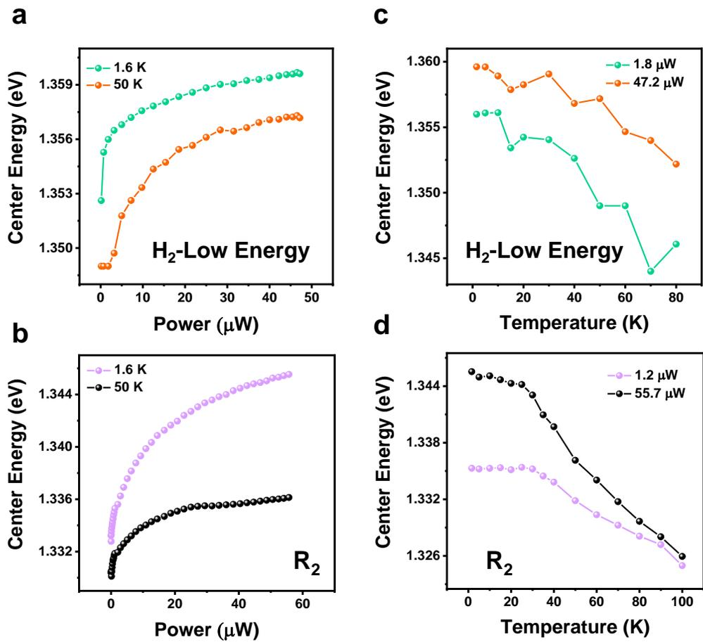
**Supplementary Fig. 2| Center energy as function of temperature and power. a-b,** Center energy as a function of power for  $\text{H}_2$  and  $\text{R}_2$  with fixed temperature (1.6 K and 50 K). **c-d,** Center energy as a function of temperature for  $\text{H}_2$  and  $\text{R}_2$  with fixed powers ( $\sim 1 \mu\text{W}$  and  $\sim 50 \mu\text{W}$ ).
