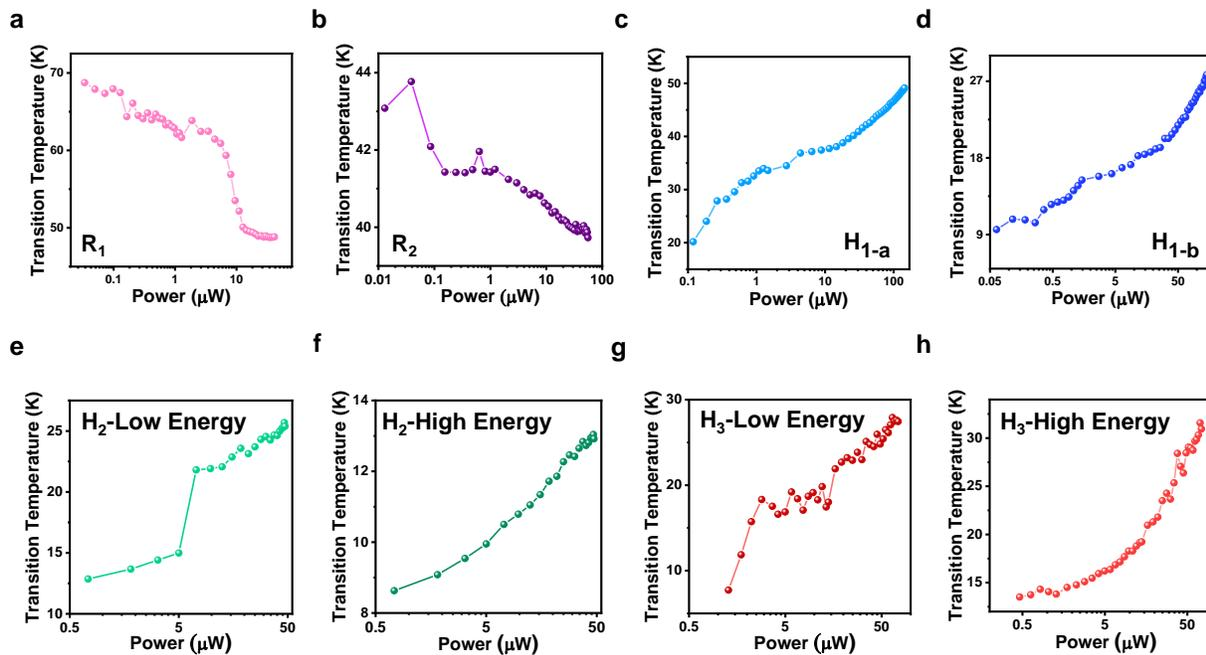
**Supplementary Fig. 5 | Power dependent transition temperature on all samples. a-h,** Transition temperature as a function of power plotted on a semi-log scale.
