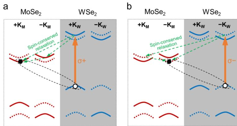
**Supplementary Fig. 7 | Spin-conserved relaxation process from intralayer exciton to IX. a,  $\sigma+$  and b,  $\sigma-$  circularly polarized excitations, which generate  $+K_W$  and  $-K_W$  intralayer excitons in  $WSe_2$ , respectively.**
