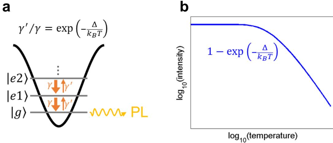
**Supplementary Fig. 9** **a**, Depiction of ground and excited states of a harmonic trap.  $\Delta$  is the effective level spacing  $\gamma$  and  $\gamma'$  are the scattering rates. **b**, Ground state IX density as a function of temperature.
