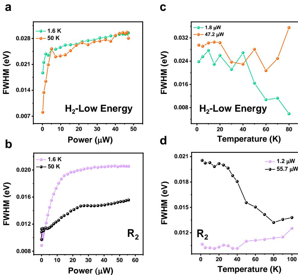
**Supplementary Fig. 3** | IX linewidth as a function of temperature and power. **a-b**, Linewidth (full width half max-FWHM) as a function of power for  $\text{H}_2$  and  $\text{R}_2$  with fixed temperature (1.6 K and 50 K). **c-d**, Linewidth (FWHM) as a function of temperature for  $\text{H}_2$  and  $\text{R}_2$  with fixed powers ( $\sim 1 \mu\text{W}$  and  $\sim 50 \mu\text{W}$ ).
