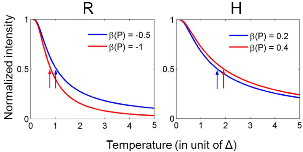
**Supplementary Fig. 10** **a**, Theoretical IX PL intensity for two different values of  $\beta$  for R-type structure showing the decreasing transition temperature with increasing power. **b**, Theoretical IX PL intensity for two different values of  $\beta$  for H-type structure showing the increasing transition temperature with increasing power.
