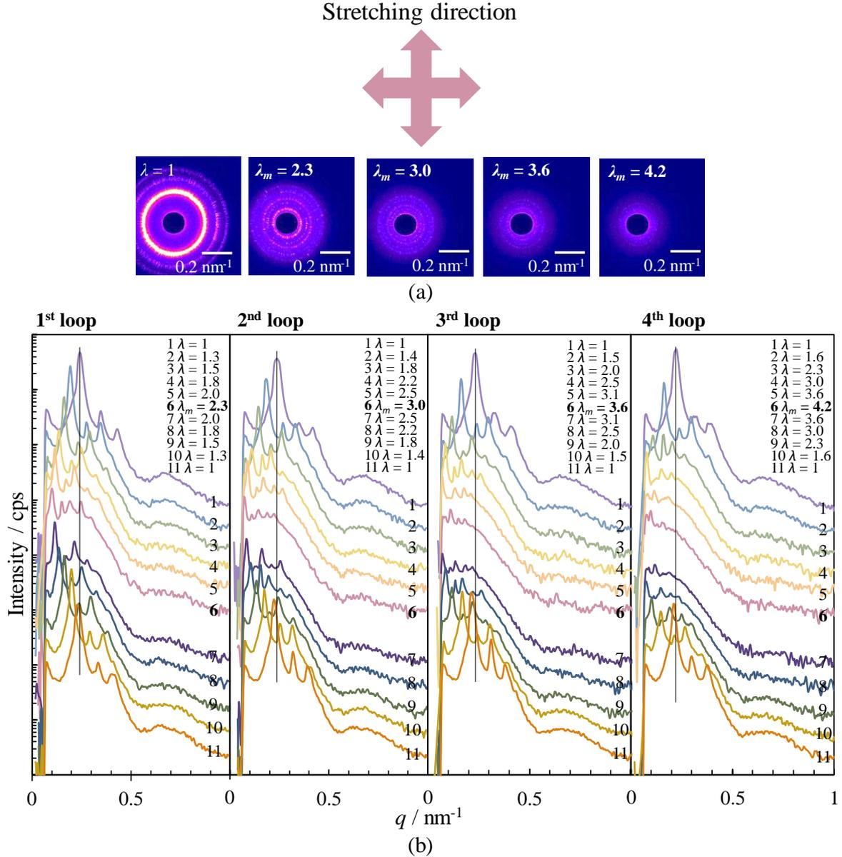
**Figure 6.** (a) 2D SAXS patterns and (b) 1D SAXS profiles of SEBS obtained from (a) in X-axis during cyclic equi-biaxial stretching at 1 mm s<sup>-1</sup> and 25°C at various  $\lambda$ s.
