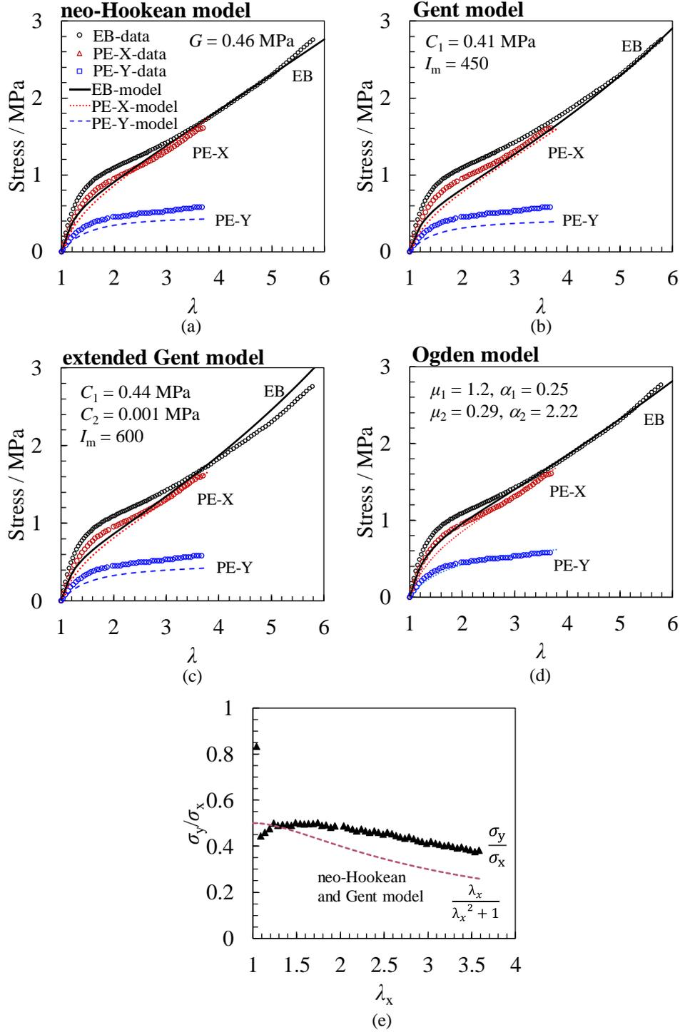
**Figure 2.** Relationships between real  $\lambda$  and stress of SEBS during equi-biaxial stretching and planar extension. Line curves correspond to the prediction of (a) neo-Hookean model, (b) Gent model, (c) extended Gent model and (d) Ogden model. (e) Stress ratio ( $\sigma_y/\sigma_x$ ) as a function of  $\lambda_x$  in planar extension of SEBS. The dashed line is the prediction of the neo-Hookean and Gent model.
