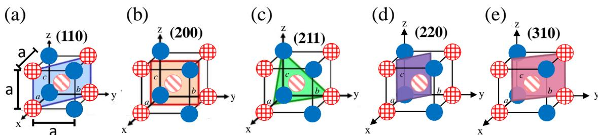
**Figure 9.** Schematic illustration of an arrangement of PS domains in (a) (110), (b) (200), (c) (211), (d) (220) and (e) (310) crystal planes of bcc lattice.
