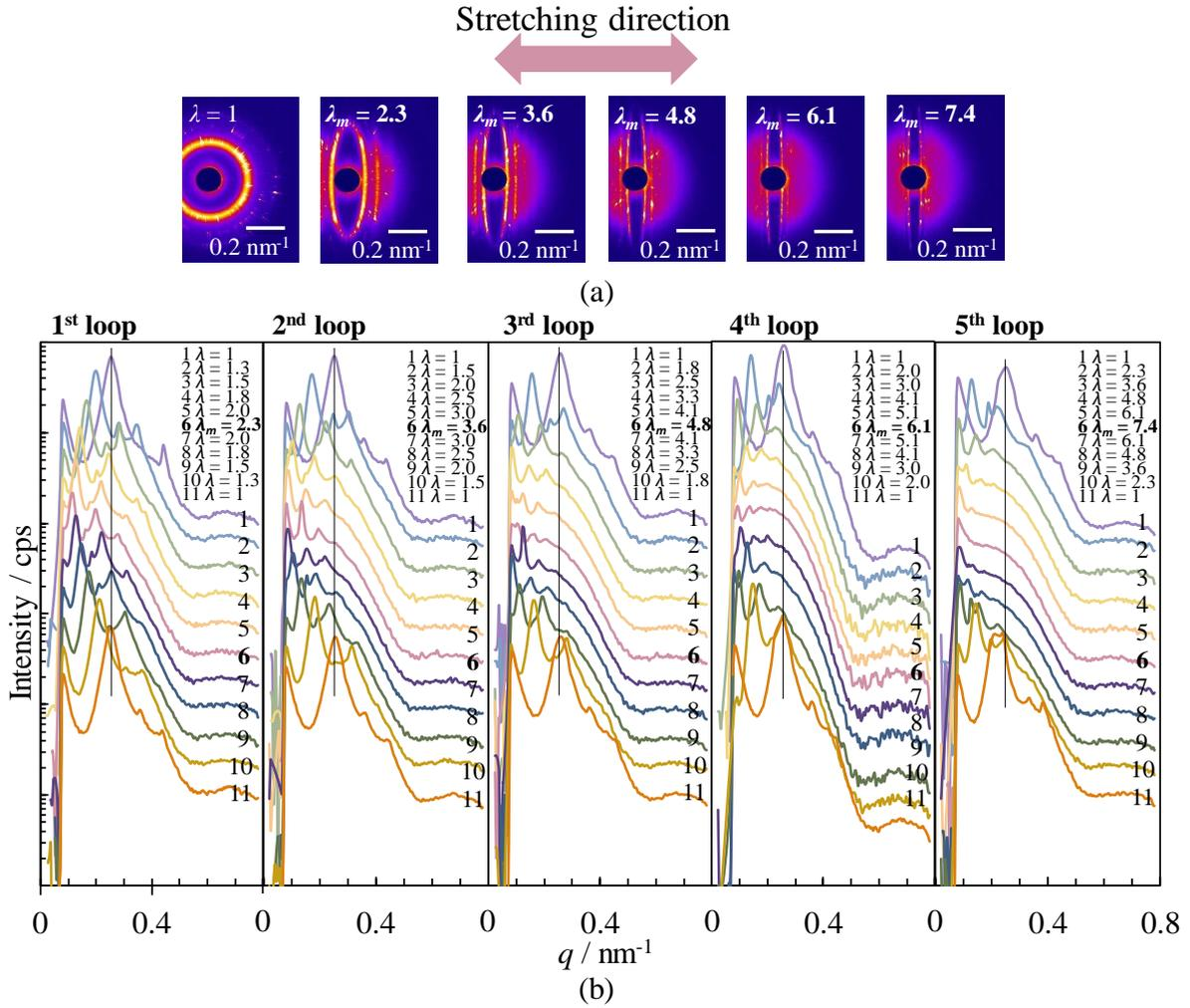
**Figure 5.** (a) 2D SAXS patterns and (b) 1D SAXS profiles of SEBS obtained from (a) in the stretching direction during cyclic uniaxial stretching at  $1 \text{ mm s}^{-1}$  and  $25^\circ\text{C}$  at various  $\lambda$ s.
