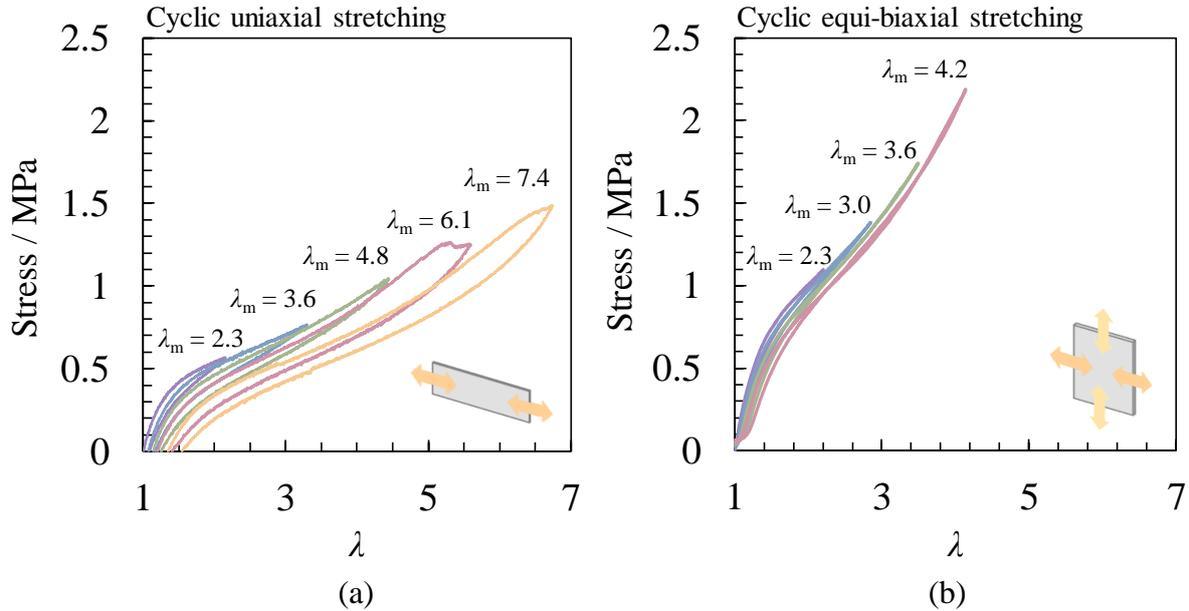
**Figure 3.** Stress- $\lambda$  relationship of SEBS under (a) cyclic uniaxial stretching and (b) cyclic equi-biaxial stretching at  $1 \text{ mm s}^{-1}$  and  $25^\circ\text{C}$ .
