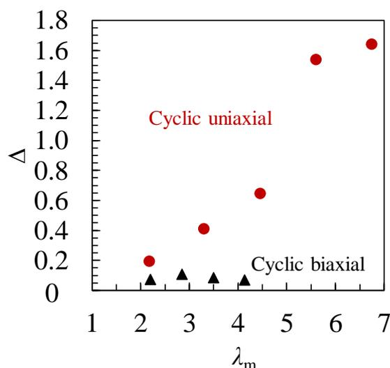
**Figure 4.** Relationship between dissipation factor ( $\Delta$ ) and  $\lambda_m$  of each cycle during cyclic uniaxial and equi-biaxial stretching at  $1 \text{ mm s}^{-1}$ .
