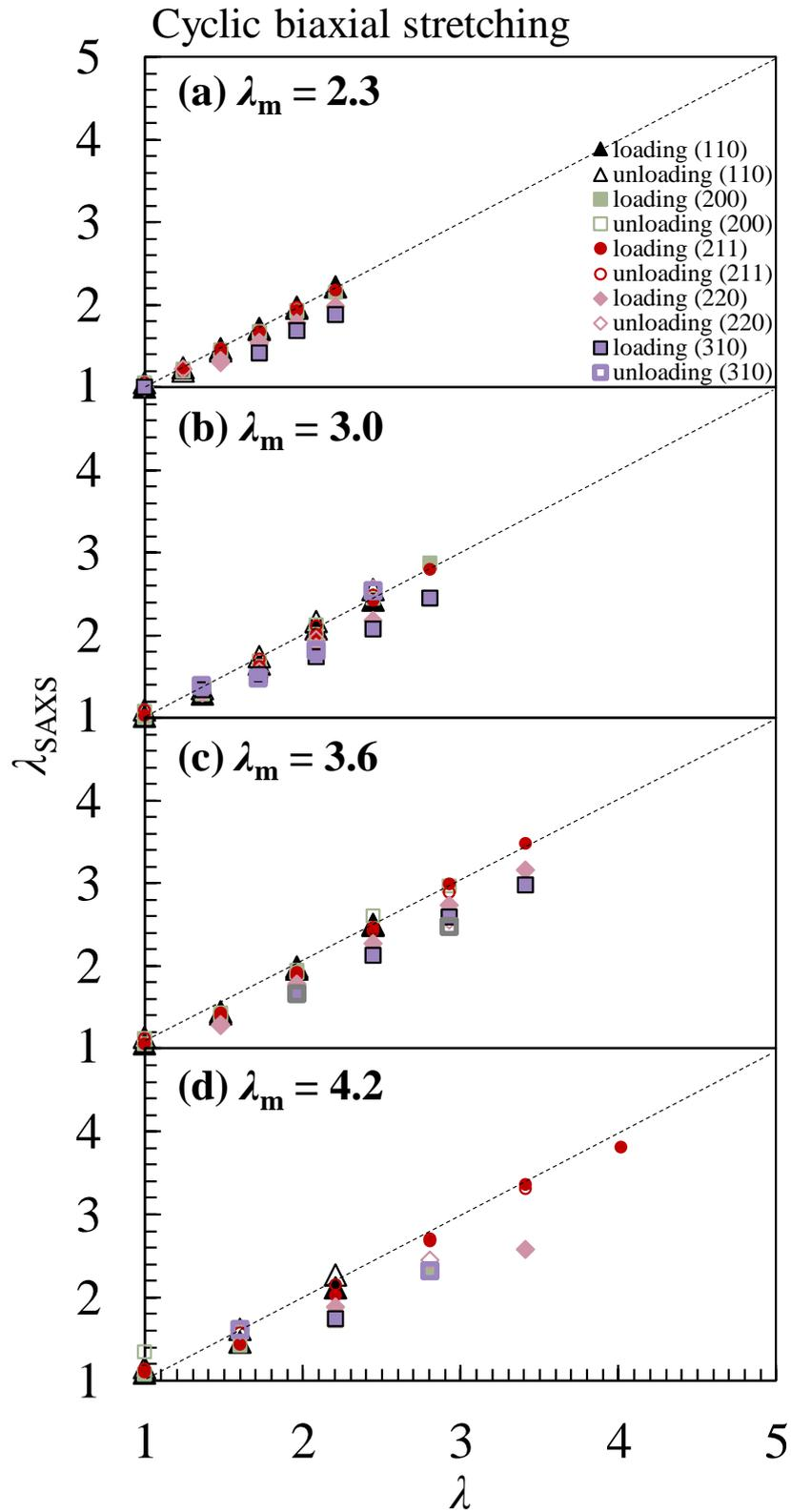
**Figure 8.** Relationship between  $\lambda$  and  $\lambda_{\text{SAXS}}$  with various  $\lambda_m$ s of (a) 2.3, (b) 3.0, (c) 3.6, and (d) 4.2 of each cycle during cyclic equi-biaxial stretching at  $1 \text{ mm s}^{-1}$ .
