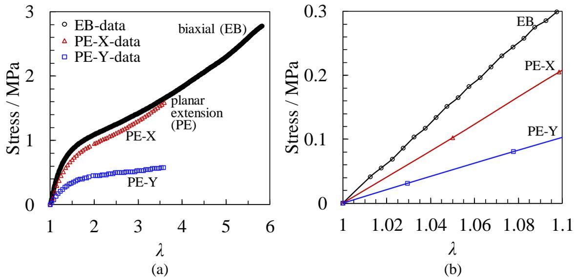
**Figure 1.** (a) Relationships between  $\lambda$  and stress of SEBS during equi-biaxial stretching and planar extension (experimental data). (b) Data of (a) at small deformation region.
