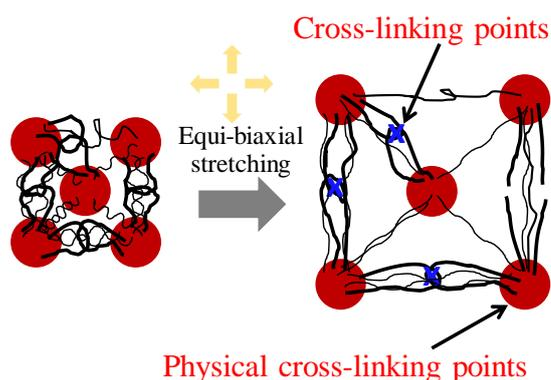
**Figure 10.** Schematic illustration of the occurrence of nominal cross-linking points during equi-biaxial stretching.
