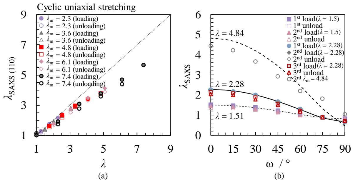
**Figure 7.** Relationship between (a)  $\lambda$  of SEBS and  $\lambda_{\text{SAXS}(110)}$  with various  $\lambda_{\text{ms}}$  during cyclic uniaxial stretching at  $1 \text{ mm s}^{-1}$ , (b)  $\lambda_{\text{SAXS}}$  with various  $\omega$ s during cyclic uniaxial stretching at  $1 \text{ mm s}^{-1}$ . Line plots are the theoretical curves of the affine deformation.
