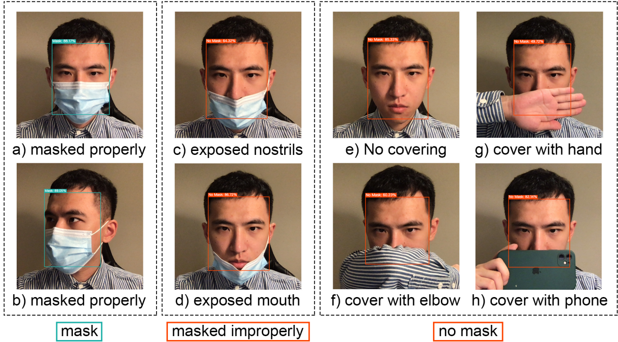
Fig. 3. This figure shows the different detection results. a) and b) show the cases with wear masks properly, c) and d) are the examples that wear mask improperly, and e), f), g) and h) are the cases of not wearing the mask.
