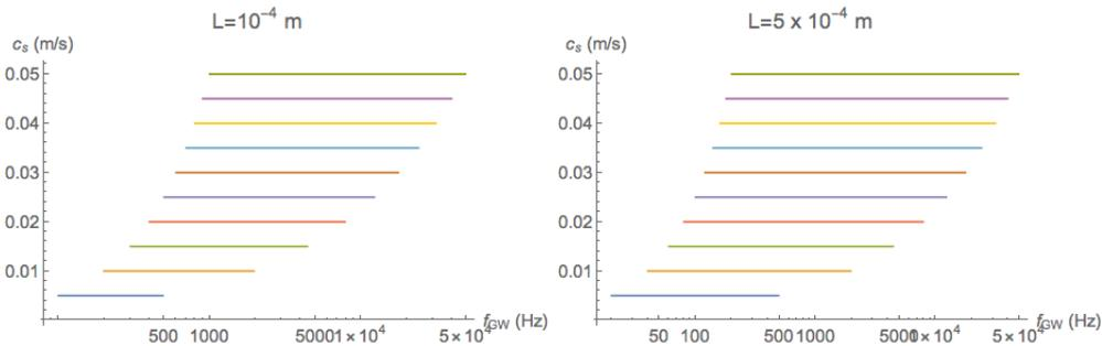
Figure 4: Frequency regime of a BEC gravitational wave detector for  $^{39}\text{K}$  atoms. Note that the larger condensates can probe lower-frequency gravitational waves, whereas those with faster speeds of sound can probe higher-frequency gravitational waves.
