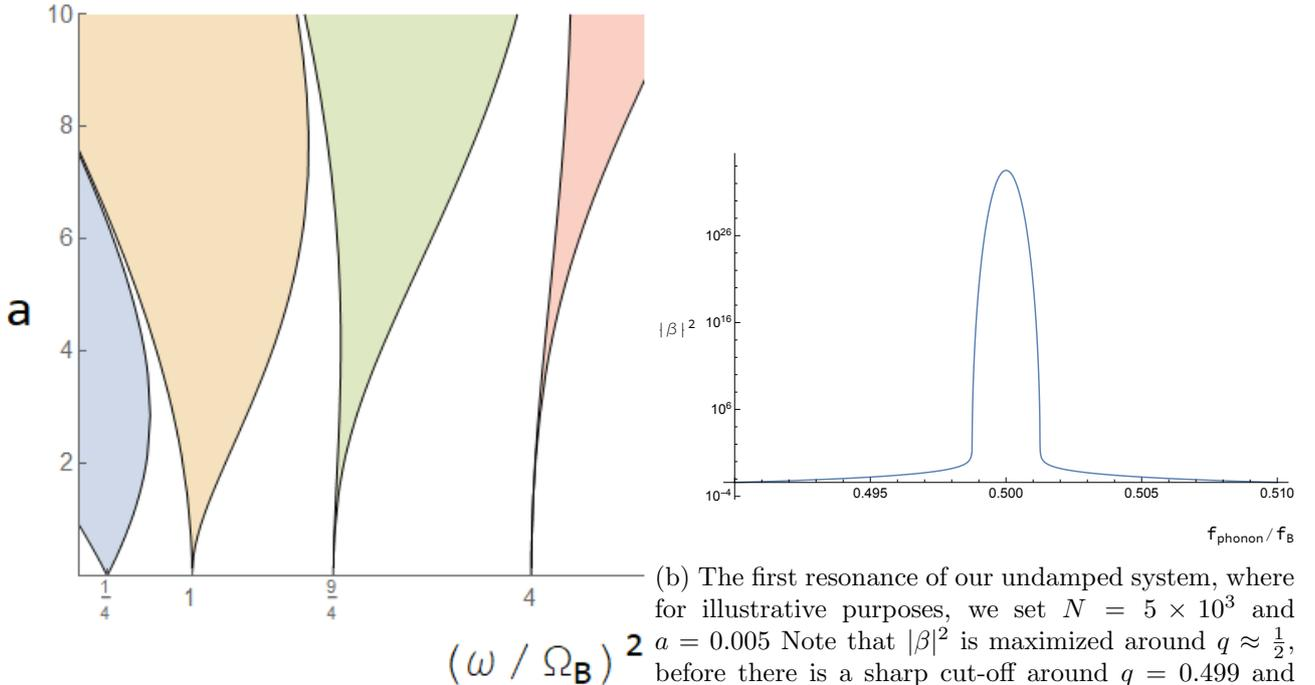
(a) Shaded areas show the locations of instability bands in  $(a, \omega)$  plane, associated with resonances of equation (11) with  $\Omega_B = \Omega$ . By lying within these regions for a time  $t$ , it is possible to improve the sensitivity to gravitational waves. Note that maximum value of  $\omega$  will be constrained by the chemical potential of the condensate.
