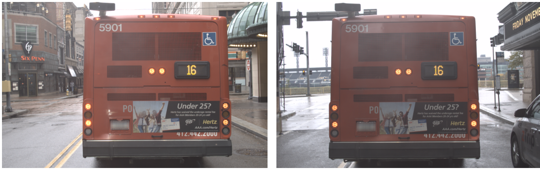
Fig. 19: Example where stereo-only loop detection fails due to the presence of the same large bus in two geographically distant frames. This sample is from the training set sequence titled day_rain_7 .
