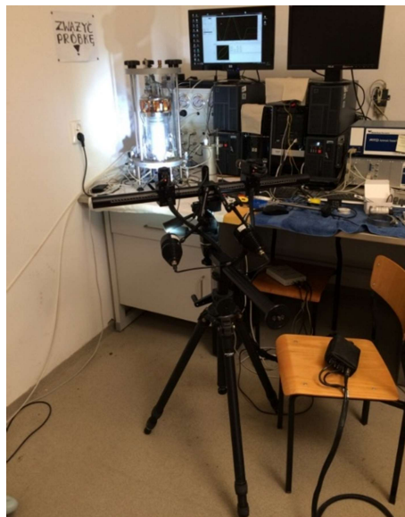
Figure 2. The specimen in TS apparatus directly illuminated with LED lamp to focus the camera.
