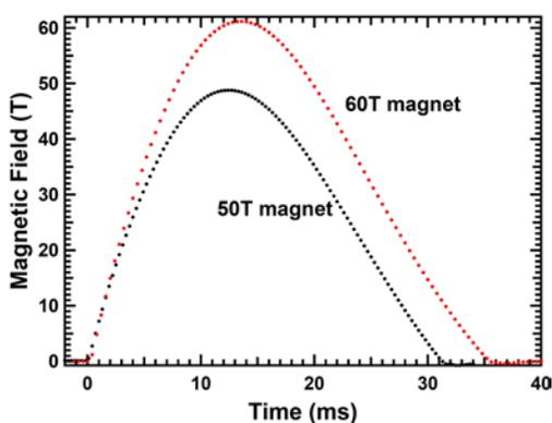
Figure S2. Pulsed magnetic field profiles used for this study. The total transient time of the fields are 31 ms and 35 ms for 50 T and 60 T magnets, respectively. Photoluminescence spectra were taken at each point, which is  $400 \mu\text{s}$  acquisition time by using an EMCCD.
