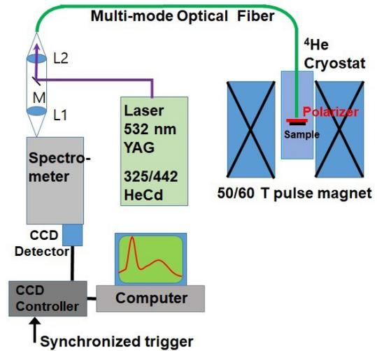
Figure S1. Experimental setup for photoluminescence under pulsed magnetic fields.
