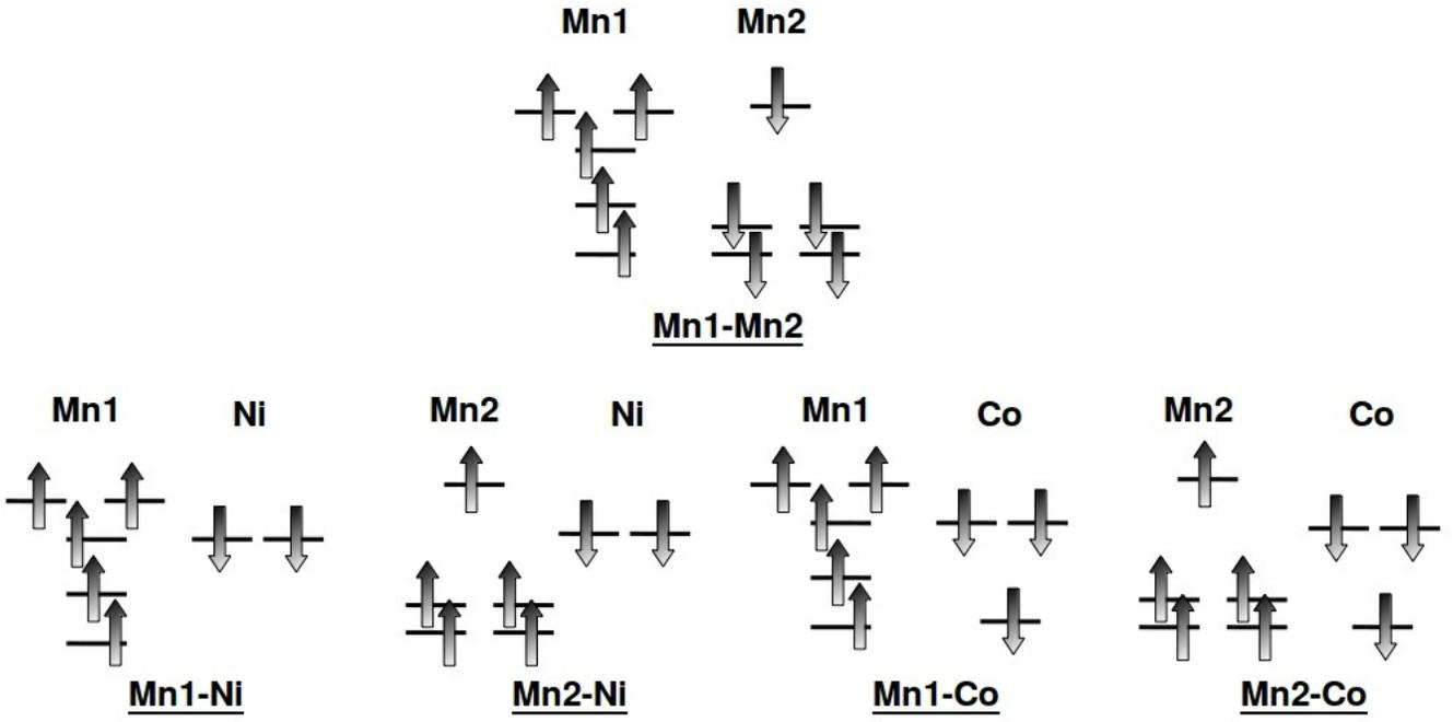
FIG. 4: Super-exchange interactions in CMNRO and CMCRO between half-filled  $d$  states of Mn1, Mn2, half-filled  $e_g$  states of Ni and half-filled  $e_g$  and one of the  $t_{2g}$  states of Co. The fully filled levels not contributing in super-exchange are not shown.
