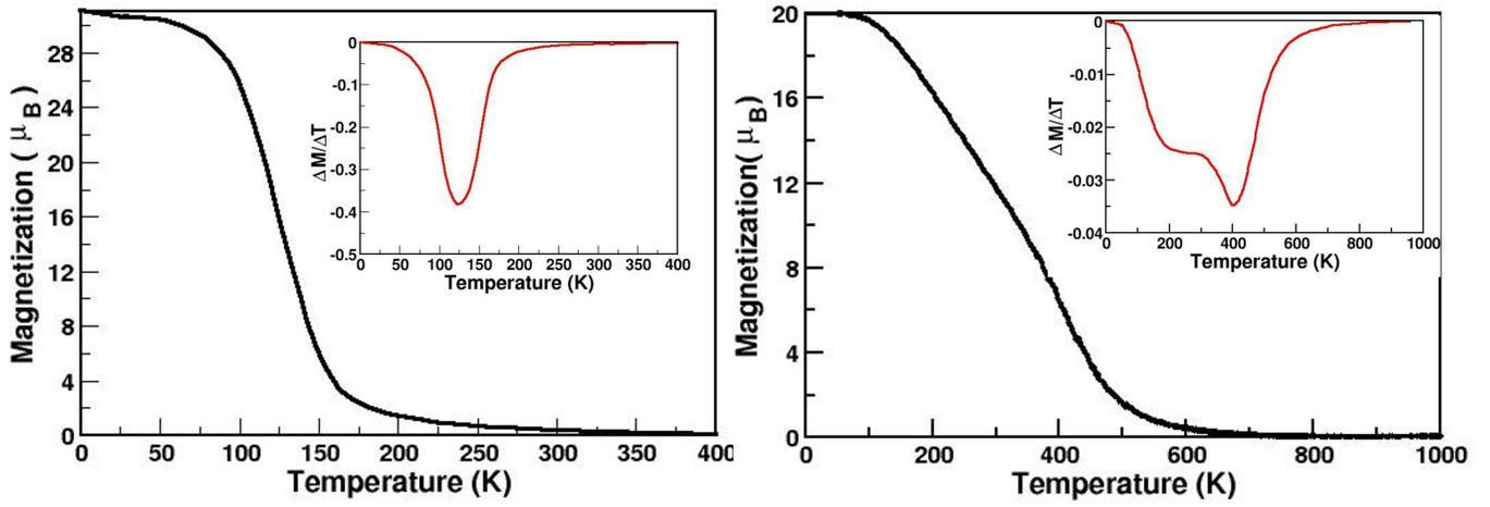
FIG. 6: (Color online) Magnetic properties of  $\text{CaMn}_{1.25}\text{Ni}_{0.75}\text{ReO}_6$  (left) and  $\text{CaMn}_{0.75}\text{Co}_{1.25}\text{ReO}_6$  (right) obtained from Monte-Carlo simulation. Insets show the derivative of magnetization as a function of temperature.
