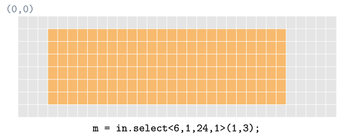
Fig. 2. Select a 6x24 sub-matrix from a 8x32 matrix
