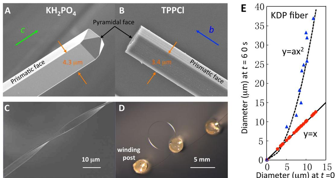
Fig. 3 **Images of single-crystalline organic and inorganic nonlinear crystal fibers.** Both KDP (A) and TPPCI (B) show prismatic face growth suppression (diameter remain unchanged) whereas the growth of pyramidal faces is unimpeded. They exhibit remarkable mechanical flexibility for twisting (C) and winding (D) (winding posts are optical fibers). (E) Prismatic face growth suppression (red dots) and quadratic growth characteristics of fibers with imperfections (blue triangles).
