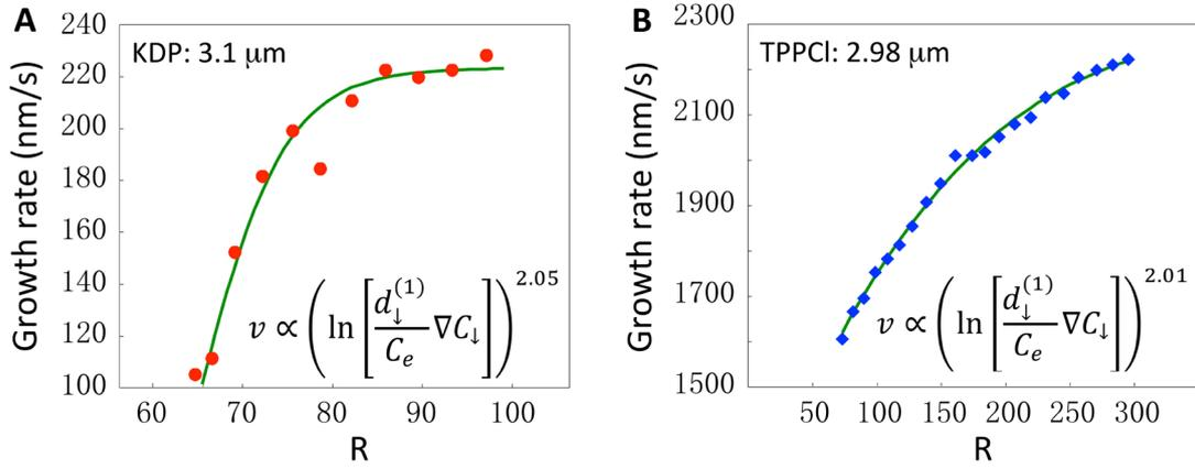
Fig. 2 **Self-channeling-stimulated growth acceleration effect.** Pyramidal face growth rate as a function of fiber aspect ratio  $R$  for KDP (A) and TPPCI (B) single-crystalline fibers subjected to prismatic face growth suppression. Green curves are fits using Eq. (1).
