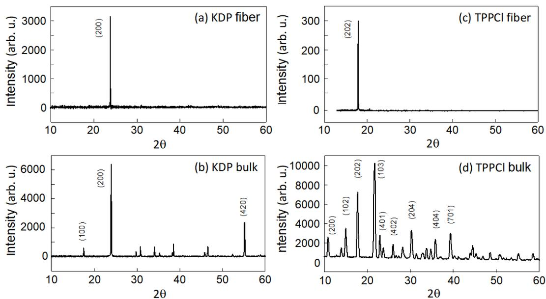
**XRD spectra of single crystal KDP (A, B) and TPPCI (C, D).**
