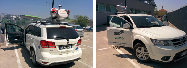
Fig. 11. SINECO S.p.A experimental vehicle equipped with RIEGL VMX-450 measurement system
