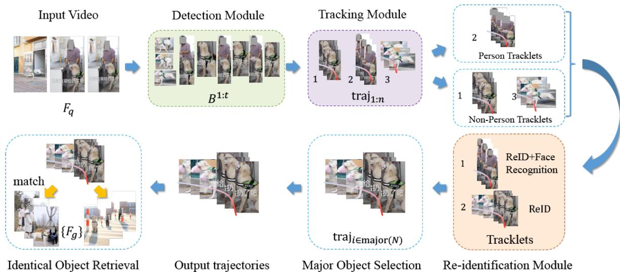
Figure 1: Overview of the overall flowchart of the generic object re-identification system.
