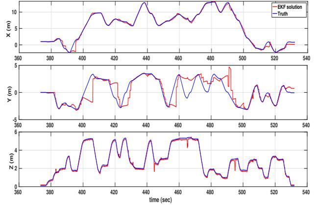
Fig. 8: In red the EKF position estimation of the best trajectory, while in blue the ground truth.
