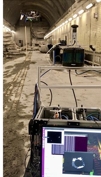
Fig. 1: Underground highway tunnel for testing purposes. In the foreground the UGV equipped with the main localization sensors and in the background the UAV flies in front of the LIDAR
