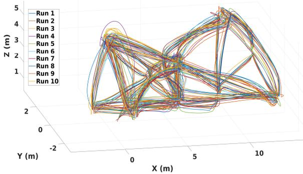
Fig. 7: UAV ground truth position of the same set of waypoints run multiple times
