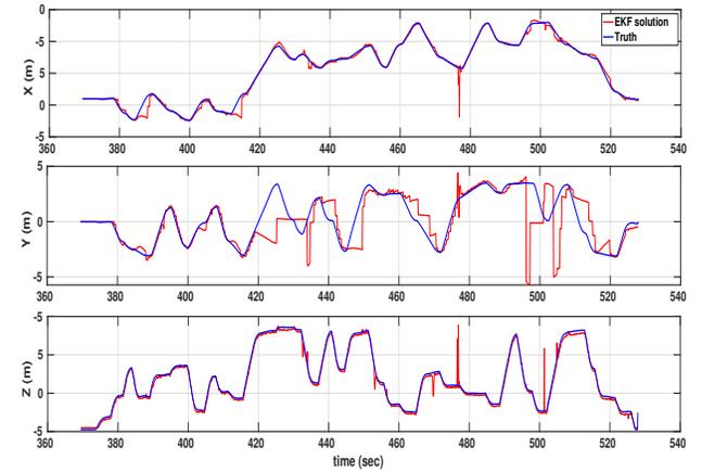
Fig. 9: In red the EKF position estimation of the worst trajectory, while in blue the ground truth.
