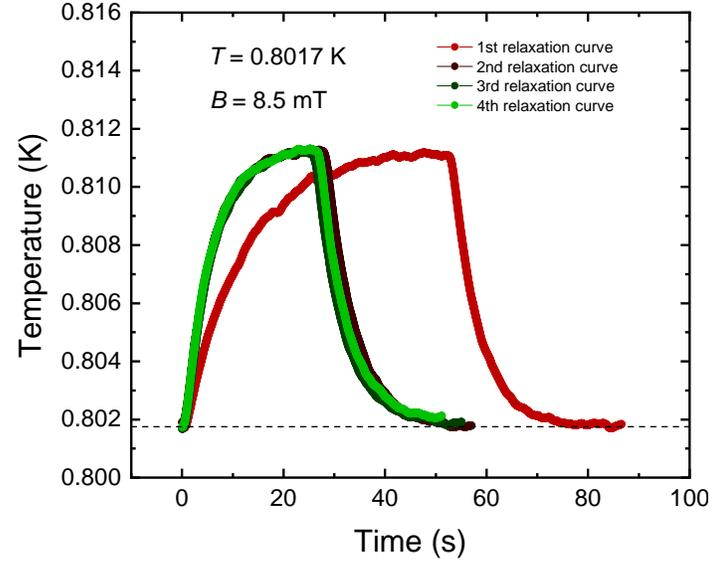
FIG. S3. Four subsequent relaxation curves at  $T = 0.802$  K and  $B = 8.5$  mT (applied after zero field cooling). The first heating curve (first part of the red solid line) reveals a longer relaxation time, implying a larger heat capacity. The cooling curve (second part of the red solid line) and all other heating and cooling curves show the same, shorter relaxation time. The effect is attributed to a change in the flux structure in the intermediate state in the first heating cycle.
