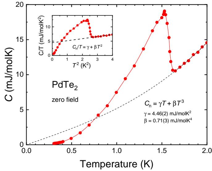
FIG. S1. As-measured specific heat of PdTe<sub>2</sub> in zero field in a plot of  $C$  versus  $T$ . The dashed line shows the normal state contribution  $C_n = \gamma T + \beta T^3$ , with the fitted values of  $\gamma$  and  $\beta$  listed in the graph. Inset: Same data in a plot of  $C/T$  versus  $T^2$ .
