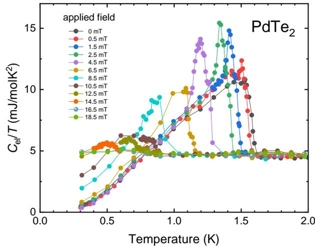
FIG. S2. Temperature variation of  $C_{el}/T$  of PdTe<sub>2</sub> in zero field and in = magnetic fields up to 18.5 mT as indicated. The increase of the step size of the specific heat at the superconducting transition temperature measured in magnetic field is clearly observed. This is due to the first order nature of the transition which involves latent heat. For  $B \geq 10.5$  mT the specific heat peak collapses.
