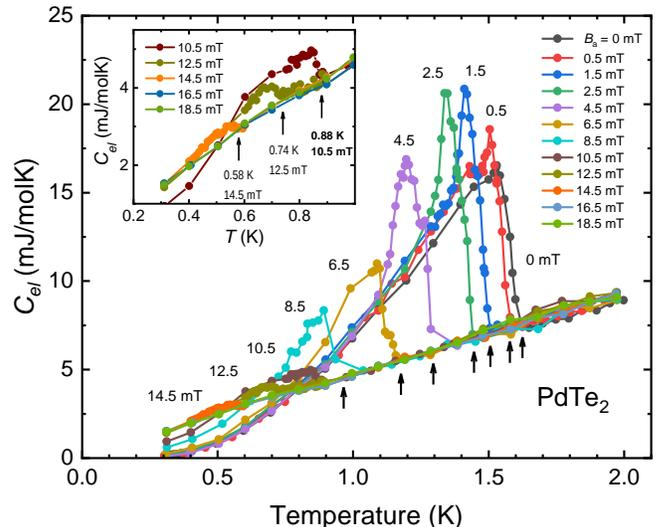
FIG. 2. Temperature dependence of the electronic specific heat  $C_{el}$  of PdTe<sub>2</sub> in zero field and in magnetic fields up to 18.5 mT as indicated. An increase in the size of the specific heat jump at  $T_c$  is observed in field.  $T_c$ 's are indicated by arrows. For  $B \geq 10.5$  mT the jump size is strongly reduced. Inset: Zoom of the data in the low temperature range for  $10.5$  mT  $\leq B \leq 18.5$  mT.
