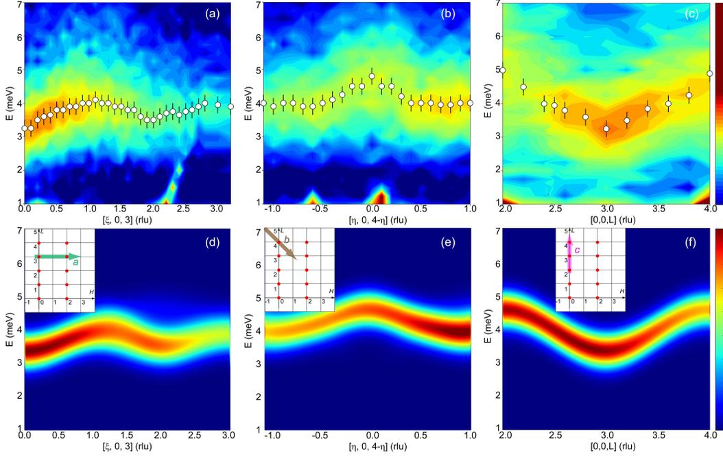
FIG. 4: SW dispersion spectra of  $\text{Tb}_2\text{Ir}_3\text{Ga}_9$  along (a)  $[\xi, 0, 3]$ , (b)  $[\eta, 0, 4 - \eta]$ , and (c)  $[0, 0, L]$ . The corresponding calculated spectra are shown in panels (d)-(f). Insets show the schematics of the scan directions in the  $(H, 0, L)$  scattering plane. The dispersion-like feature for energy transfer below 3 meV in panel (a) arises from the tail of the resolution function sweeping through the neighboring Bragg peak in the focusing geometry.
