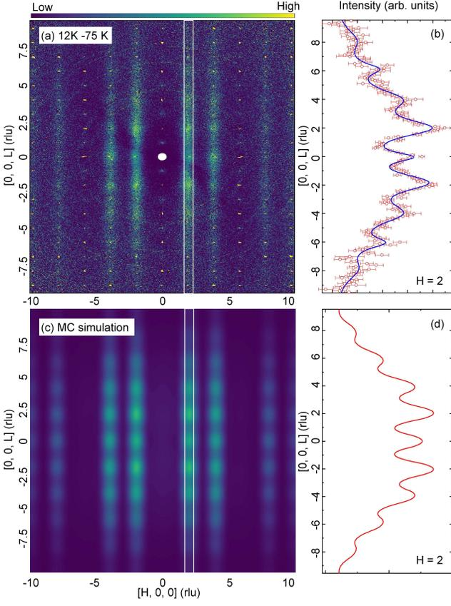
FIG. 3: (a) Contour plot of the neutron diffraction data in the  $(H, 0, L)$  scattering plane. A rod-like feature along  $[0, 0, L]$  indicates the short-range magnetic correlations along the  $c$  axis. (b) For the line cut along  $[2, 0, L]$ , Lorentzian profiles appear at even indices. (c) Monte-Carlo simulation of the magnetic diffuse scattering just above the transition using the magnetic exchange parameters in Tab. II. (d) The corresponding line cut along  $[2, 0, L]$ .
