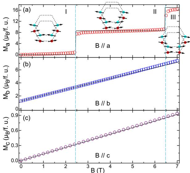
FIG. 5: Magnetization  $M(H)$  with field applied along the three crystallographic axes up to 7 T at 1.8 K. Open symbols are experimental data; solid lines are the best fits described in the text. The spin configurations in three distinct region with field  $B \parallel \mathbf{a}$  are sketched in panel (a).
