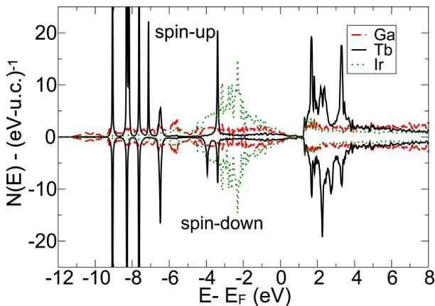
FIG. 6: The calculated density-of-states of  $\text{Tb}_2\text{Ir}_3\text{Ga}_9$  in the  $\text{AF}_1$  phase.
