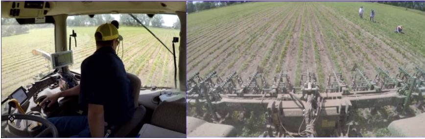
Fig. 1. (Left) An operator in a semi-automated tractor. (Right) A RoboCrop Cultivator Head running in a field of beets. Note the H2A workers outside the path of the tractor on the right.
