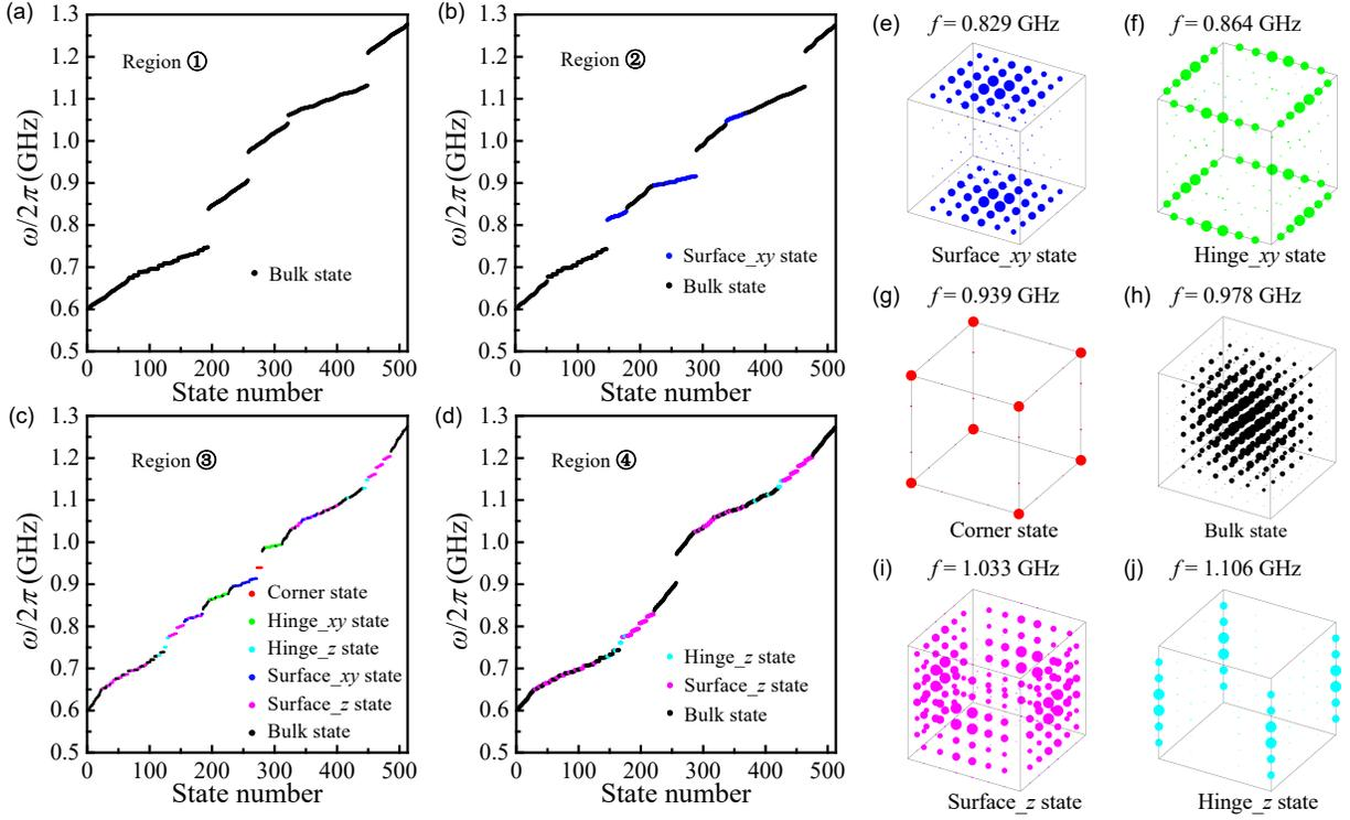
FIG. 3: Eigenfrequencies of the collective vortex gyration in a three-dimensional  $8 \times 8 \times 8$  system for parametric region ① (a), parametric region ② (b), parametric region ③ (c), and parametric region ④ (d), as marked in Fig. 2(b). (e)-(j) The spatial distribution of different modes. Here the size of the colorful balls is proportional to the amplitude of the wavefunction.
