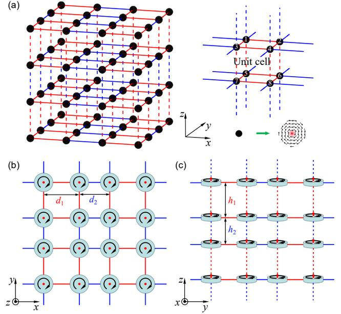
FIG. 1: (a) Illustration of a three-dimensional magnetic vortex lattice, with black balls denoting nanodisks with vortex state and solid (dashed) red and blue segments representing alternating lengths of intralayer (interlayer) intracellular and intercellular bonds, respectively. Top (b) and side (c) view of the crystal structure.  $d_1$ ,  $d_2$ ,  $h_1$ , and  $h_2$  are the bond lengths.
