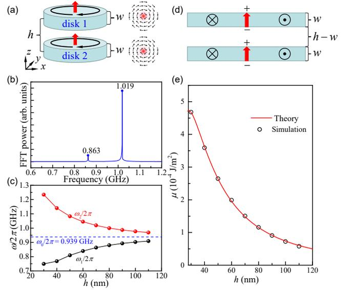
FIG. 6: (a) Schematic plot of the stacking two-vortex system. The micromagnetic structures of vortices are also shown. (b) The Fourier spectrum of the vortices oscillation for  $h = 70$  nm. (c) The two eigen frequencies of the two-vortex system varying with  $h$ . (d) The illustration of the interaction between magnetic charges. (e) Dependence of the interlayer coupling parameter  $\mu$  on  $h$ . Black circles denote simulation results and red solid line represents the analytical formula.
