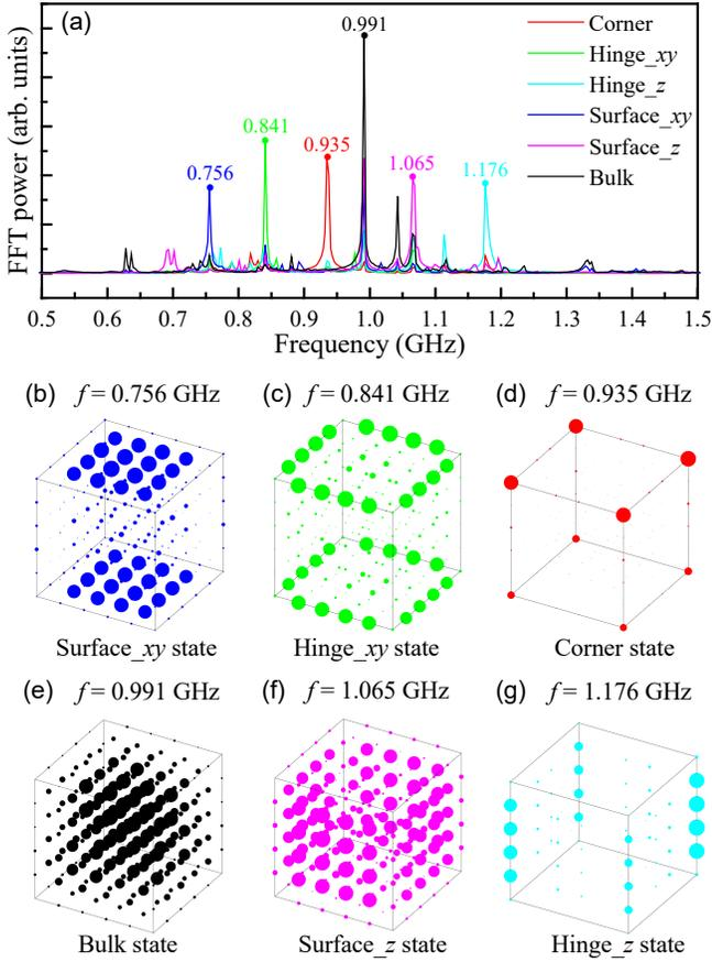
FIG. 4: (a) The temporal Fourier spectra of the vortex oscillations at different positions. (b)-(g) The spatial distribution of FFT intensity with different frequencies as marked in (a). The size of the balls reflects the strength of the oscillation.
