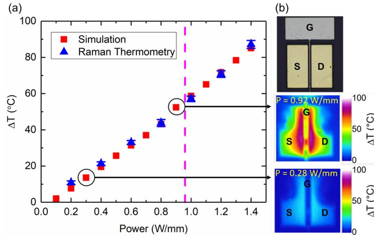
**Fig 5:** (a) The channel temperature rise determined by Raman thermometry and thermal modeling. The pink dashed line corresponds to the current inflection point shown in Fig. 3(a). (b) Optical image of the device under test and 2D temperature maps generated by IR thermal microscopy corresponding to power densities of 0.92 W/mm and 0.28 W/mm.
