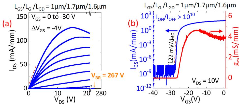
**Fig 3:** (a) Output characteristics and (b) Transfer characteristics of fully MOVPE-grown  $\beta$ -Ga<sub>2</sub>O<sub>3</sub> MESFET with regrown S/D contacts.
