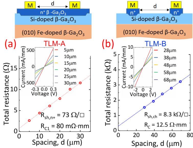
**Fig 2:** Schematic of TLM structure, corresponding IV plots (inset) and total resistance vs contact spacing plots of (a) TLM pads on the MOVPE-regrown  $n^+$   $\text{Ga}_2\text{O}_3$  region and (b) TLM pads with patterned MOVPE-regrown  $n^+$  ohmic contacts.
