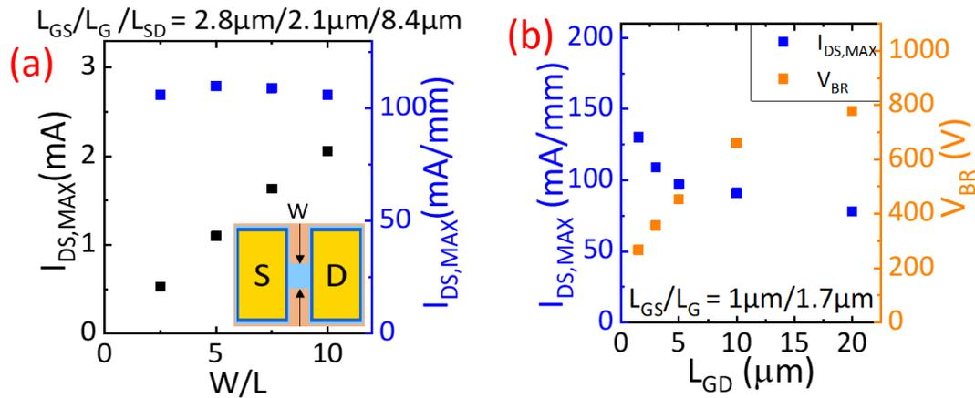
**Fig 4:** (a)  $I_{DS,MAX}$  for devices with different channel width to length ratios ( $W/L$ ) (b)  $I_{DS,MAX}$  and  $V_{BR}$  of devices with different  $L_{GD}$ .
