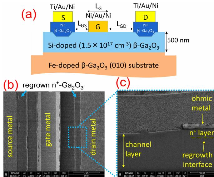
**Fig 1:** (a) Schematic of the fully MOVPE-grown Ga<sub>2</sub>O<sub>3</sub> MESFET with regrown ohmic contacts. (b) Top view SEM image of the MESFET showing the regrown access regions. (c) Cross-sectional SEM of the contact region showing the estimated regrowth interface.
