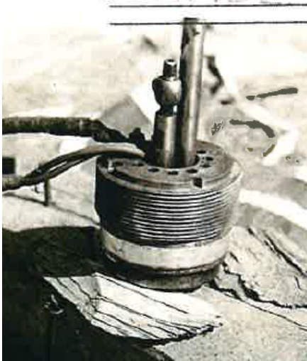
Figure 14. A Jumbino closure assembly showing lead wires, gas release valve, and bottom of pressure gauge, circa late 1944.
