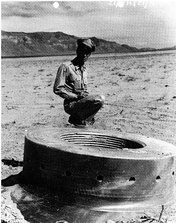
Figure 34. The Jumbo nozzle forging laying on the desert floor after the Army experiment, April 16, 1946. Note the diameter and threading of the nozzle.
