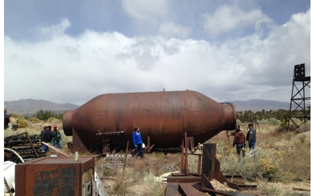
Figure 40. Jumbo #3 resting on the side of the PHERMEX firing point, May 1, 2014. Note the field-welded legs that may have created new damage to the vessel. History repeats itself.
