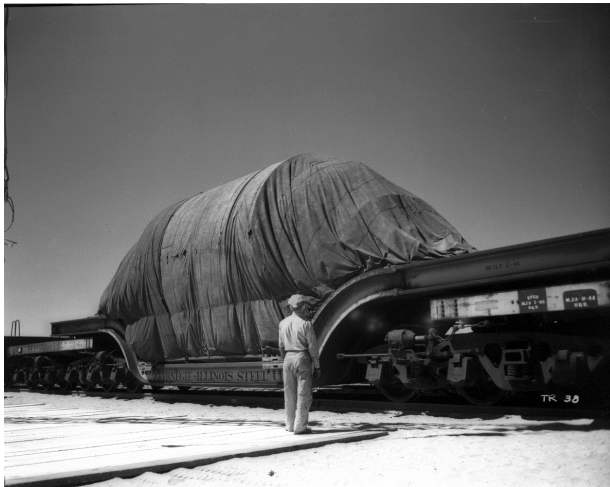
Figure 24. CISX 500 with a 214-ton “Straight Length Banded Accumulator” strapped and covered with a large tarpaulin, circa 1945.
