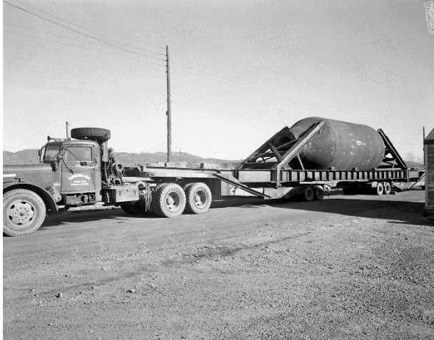
Figure 336. Lowdermilk Bros. Construction Company's overloaded trailer in Santa Fe, NM on January 24, 1952. Note the additional structure welded to Jumbo #3 to stabilize the load.
