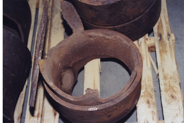
Figure 15. Laminated remnants of a Jumbino tested to failure. Picture taken in Aug 2004.
