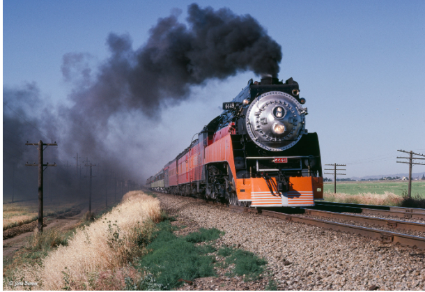
Figure 23. Southern Pacific #4449 “Daylight, circa 1981.” Daylight is 110-feet long, 10-feet wide, and 16-feet tall. Daylight weighs 394 tons. Photo courtesy of John Benner.
