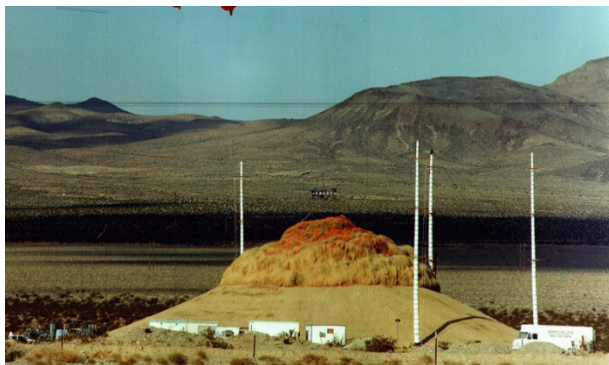
Figure 5. November 1982 Gravel Gertie shot with 423 lb HE at the Nevada Test Site 7 .
