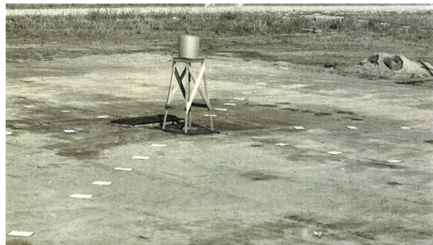
Figure 6. Initial tests of the water-capture method on an asphalt strip, circa early 1944.
