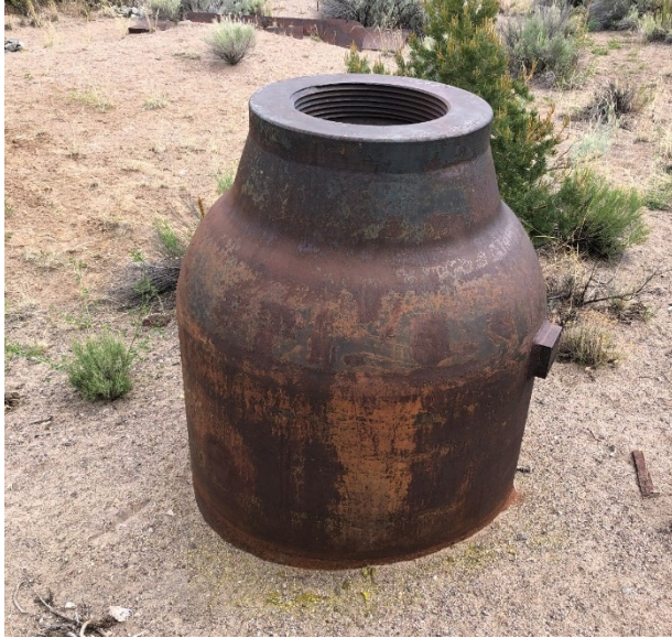
Figure 16. Dumbo resting on the IJ firing point, May 29, 2020. Note the unusual geometry of the vessel head and the uranium oxide (yellow dust) in the sand around the partially buried vessel.
