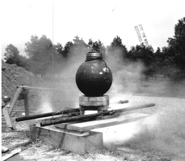
Figure 10. Cast-steel vessel failure from the bottom plug/manway, early 1944.
