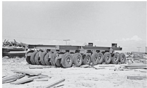
Figure 25. The Rogers-built trailer for Jumbo, 18-feet wide by 40-feet long with 64 desert-type tires. Photo is post Trinity, circa late 1945.
