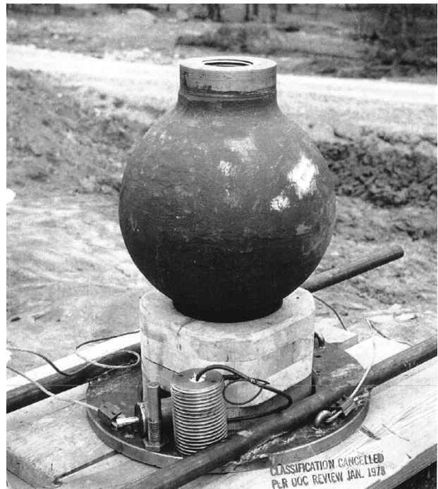
Figure 9. Cast-steel vessel test setup, early 1944. Note threaded plug with cable feedthrough.
