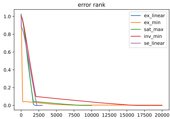
Fig. 27: Convergence plot of the different RF pulse designs using the proposed algorithm. In most cases, the algorithm will converge around 2000 iterations.
