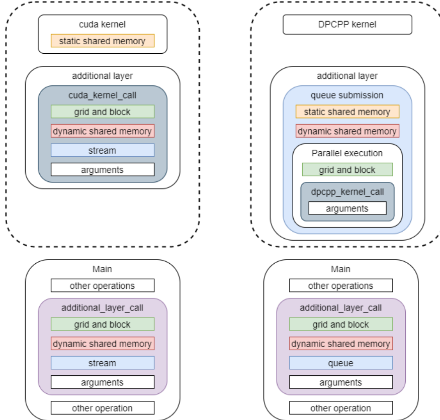
Figure 5: Wrapping the hardware-specific kernels written in HIP, CUDA, and DPC++ into an intermediate layer enables consistency in the kernel invocation across all backends.
