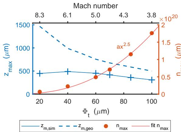
FIG. 4. Evolution of the on-axis shock position (blue cross) and of the maximum density at this point (orange dot) as a function of the throat diameter, and corresponding Mach number at the end of the diverging section. The blue dashed line represent the predictions of the geometrical model of section II. The orange line is a power fit of the maximum density data. Simulations are performed in nitrogen with a backing pressure  $P_{back} = 50 \text{ bar}$
