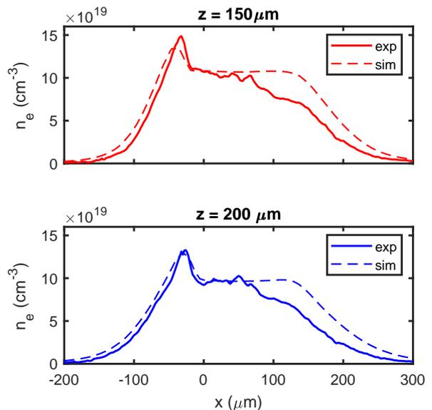
FIG. 6. Comparison of measured and simulated plasma profile obtained with a one-sided shock nozzle using nitrogen with a backing pressure of 15 bar at a distance of a)  $150 \mu\text{m}$  and b)  $200 \mu\text{m}$  from the nozzle's exit
