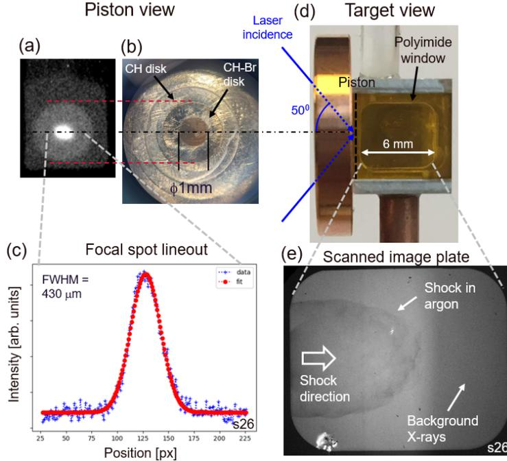
FIG. 2. (a)-(c) View of the piston: (a) X-ray emission from the laser-piston interaction from a time-integrated pinhole camera diagnostic. (b) Microscope image of the 1 mm diameter shock aperture and CH-Br / CH pistons. (c) Lineout of (a) and Gaussian fit to estimate the laser spot size. (d)-(e) Target view: Field of view of the X-ray backlighting diagnostic of a single shock target and example of raw X-ray image result respectively.
