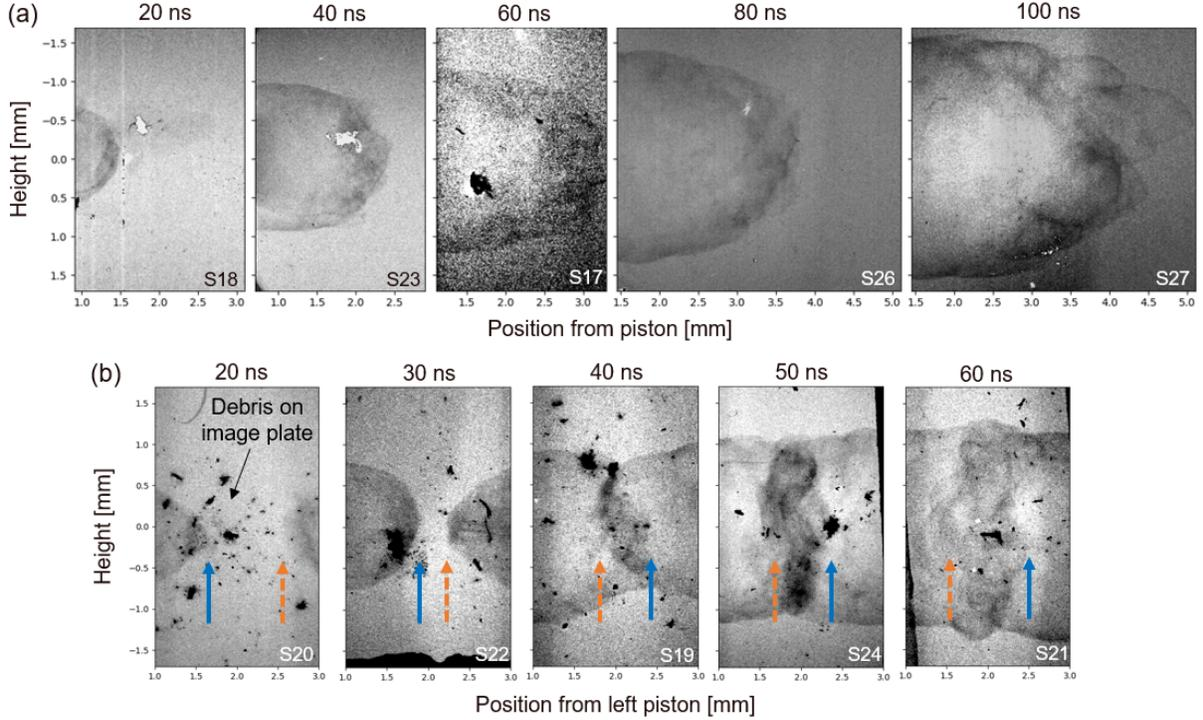
FIG. 3. X-ray backlighting results for (a) single and (b) colliding shocks. Artefacts from hard X-ray background (see Fig. 2e) have been removed for visual purposes. For colliding shocks, the position is taken relative to the left-hand side piston and the vertical arrows mark the approximate position of the shock fronts in each frame. The arrows suggest that the shocks interpenetrate however, in reality, the experiments are in a collisional regime where no interpenetration occurs.
