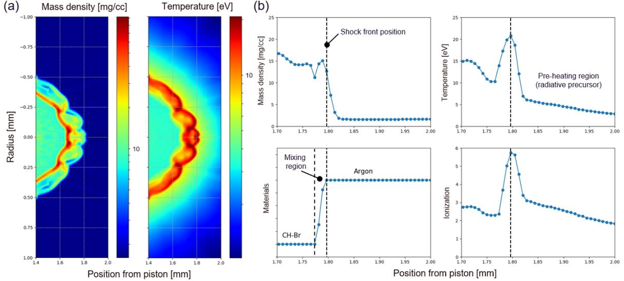
FIG. 5. Numerical simulations of the experiments with the 2-D radiation hydrodynamics code ARWEN at 20 ns. (a) Maps of mass density and temperature. (b) Axial lineouts (at a radius of 0 mm) of mass density, temperature, materials and ionization from (a).
