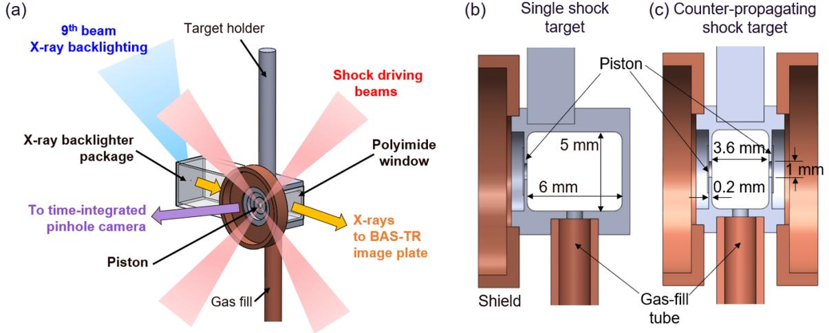
FIG. 1. (a) Schematic diagram of the experimental setup for a single shock target on the SG-II laser, with a similar configuration used for counter-propagating shocks. (b)-(c) Cross-section of single and counter-propagating shock targets.
