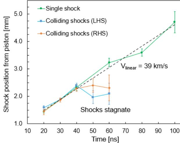
FIG. 4. Shock front position as a function of time measured from the results in Fig. 3 for single and colliding shocks. For the latter, the positions of the shock fronts are marked in Fig. 3b with matching colours.
