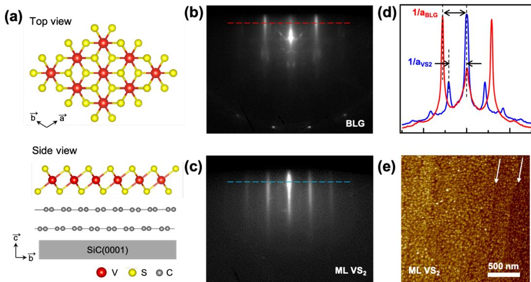
Figure 1. (a) Top- and side-view schematics of ML VS<sub>2</sub> on BLG. RHEED patterns of (b) BLG and (c) ML VS<sub>2</sub>. (d) Horizontal line profiles of RHEED patterns on BLG (red) and ML VS<sub>2</sub> (blue). (e) Topographic AFM image of the ML VS<sub>2</sub>.
