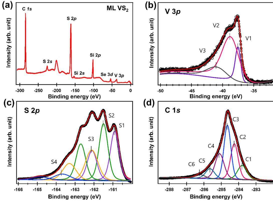
Figure 2. XPS spectra of the ML VS<sub>2</sub> at normal emission (a) wide scan, (b) V 3p, (c) S 2p, and (d) C 1s.
