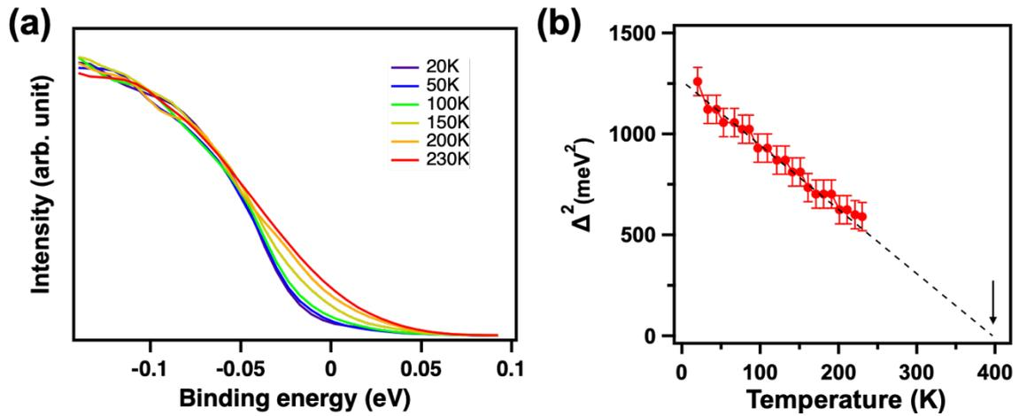
Figure 4. Temperature dependence of CDW gap of ML VS<sub>2</sub>. (a) Energy dispersive curves at the  $\Gamma$  point near Fermi energy, (b) Squared energy gap as a function of temperature along with linear fitting (black dashed line).
