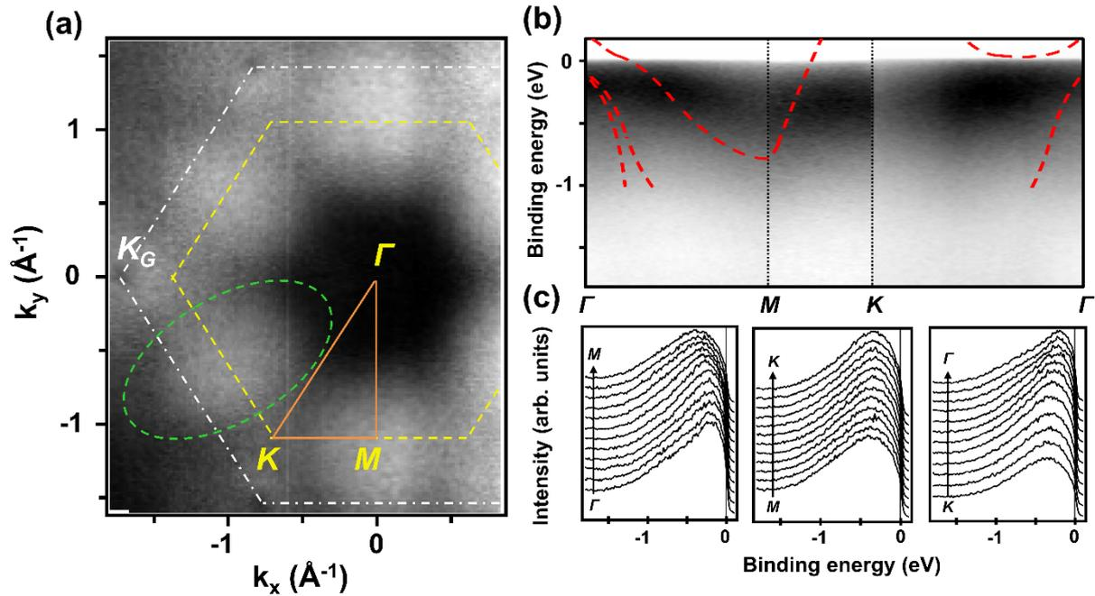
Figure 3. ARPES of ML VS<sub>2</sub>. (a) Fermi surface map with hexagonal BZ of VS<sub>2</sub> (yellow dashed line) and that of BLG (white dot-dashed lines). (b) Intensity map along the  $\Gamma$ -M-K- $\Gamma$  (orange lines in (a)) compared with the DFT band structure from the reference [49]. (c) Energy distribution curves along  $\Gamma$ -M, M-K, and K- $\Gamma$  extracted from (b).
