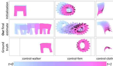
Figure 5: Visuomotor Control: \nabla Sim provides gradients suitable for diverse, complex visuomotor control tasks. For control-fem and control-walker experiments, we train a neural network to actuate a soft body towards a target image (GT). For control-cloth , we optimize the cloth’s initial velocity to hit a target (GT) (specified as an image), under nonlinear lift/drag forces.
