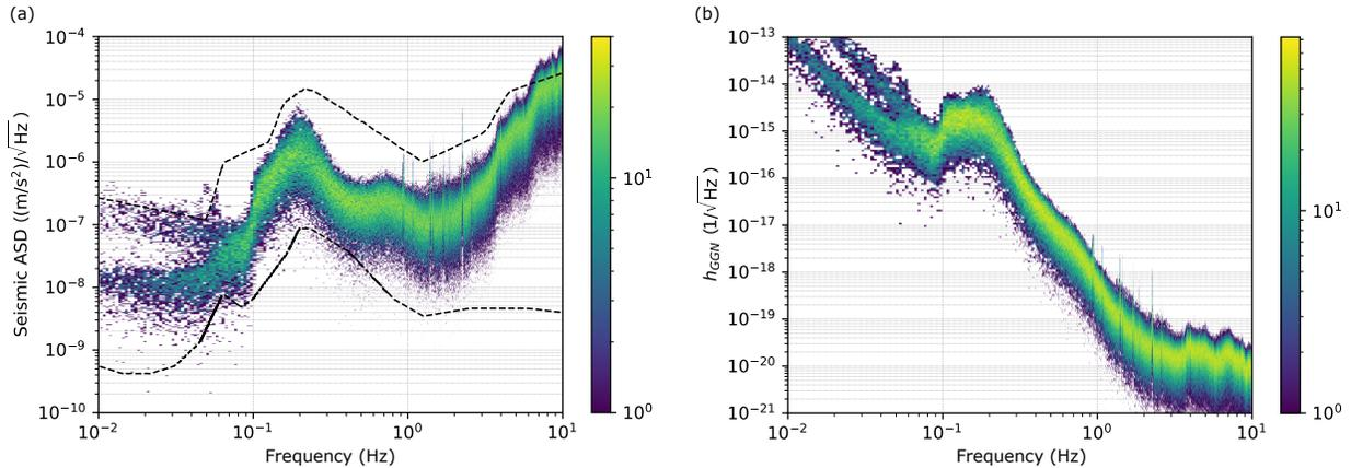
**Figure 18.** (a) Seismic acceleration amplitude spectral density for the surface of the MINOS shaft at Fermilab over a period of 30 days. Dashed black lines represent the NLNM and NHNM. (b) Inferred GGN strain amplitude spectral density modeled from surface displacement measurements. The color bar represents amplitude counts per frequency bin. All data was acquired with a sampling rate of 50 Hz.
