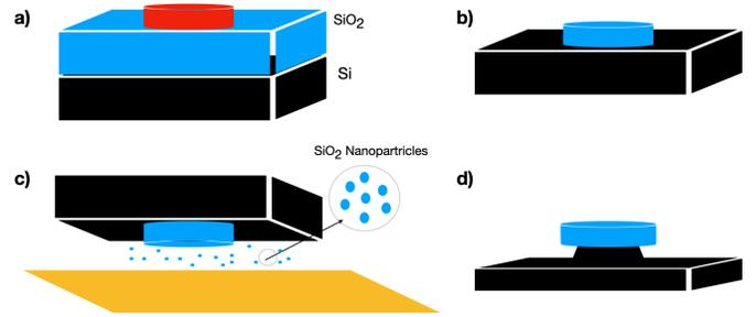
FIG. 1. a) Photolithography of the resist to transfer the pattern, b) HF wet etch to make the disk, c) CMP step to increase the smoothness of the surface, and d) etching Si substrate to make the pillar.
