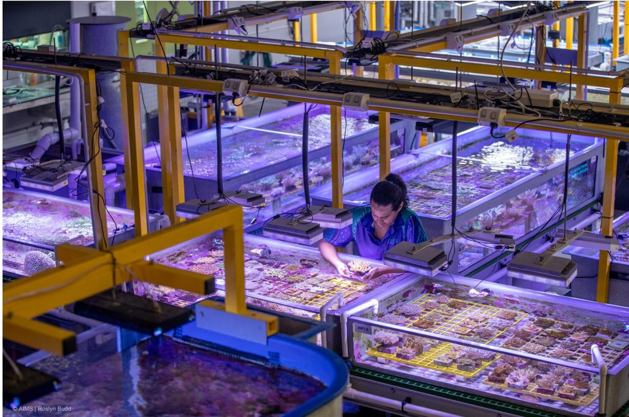
*Figure 10.* SeaSim at AIMS uses models of ocean conditions to automatically simulate conditions in tanks, in order to observe coral behaviour. Credit Roslyn Budd
