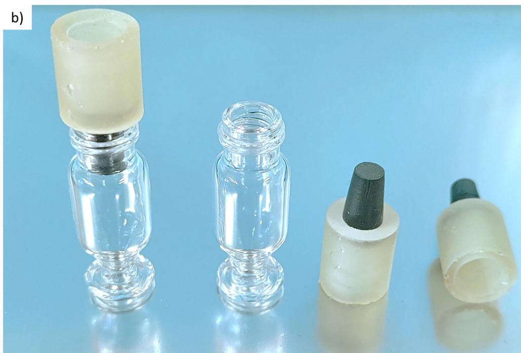
*Fig. S2: a) Cotton swap adaptor mounted onto the pipetting channel, removing a small stripe of the coated layer to contact the transparent back electrode. b) Left: 1 ml vial capped with a fluorinated rubber cork adaptor, which can be picked up by a pipetting channel of the pipetting robot. Middle and right: Bare vial and two cork adaptors.*
