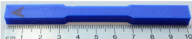
Figure 4: Example control group test specimen.
