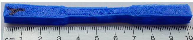
Figure 5: Example 50% material reduction.
