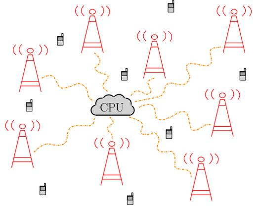
Fig. 1. Cell-free massive MIMO system.
