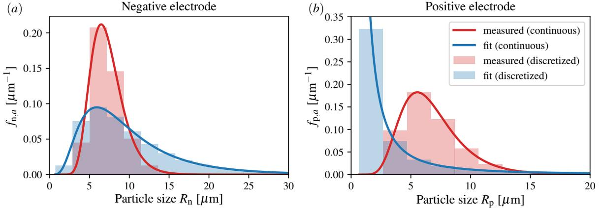
Figure 7: Area-weighted particle-size distributions  $f_{k,a}(R_k)$ ,  $k = n, p$  from direct measurements [18] (red) and from fitting the MP-DFN model to voltage relaxation data (blue). The continuous lognormal densities are shown, as well as the discrete distributions that were employed in the PyBaMM simulations. For the means ( $\bar{R}_{k,a}$ ) and standard deviations ( $\sigma_{a,k}$ ) see Table 2.
