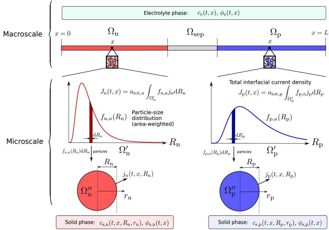
Figure 1: Schematic depicting the multi-scale geometry used for the Many-Particle-DFN model. The macroscale ( $x$ ) and microscale dimensions ( $R_k, r_k$  for  $k = n, p$ ), as well as the fundamental variables in the solid and electrolyte phases, are shown.
