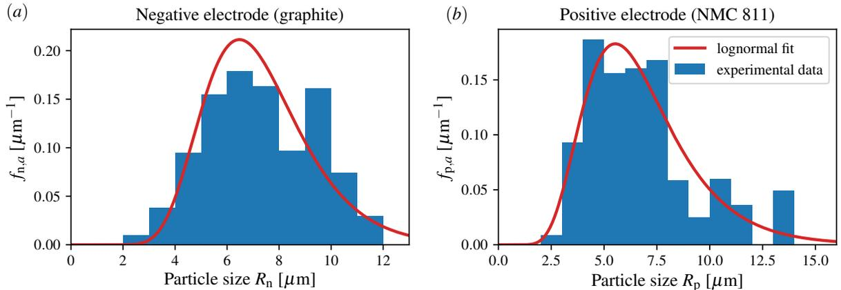
Figure 2: Experimental measurements and lognormal fits of area-weighted particle-size distributions  $f_{k,a}(R_k)$ , using data from Chen et al. [18]. (a) Negative electrode  $k = n$  (graphite only); (b) Positive electrode  $k = p$  (NMC 811).
