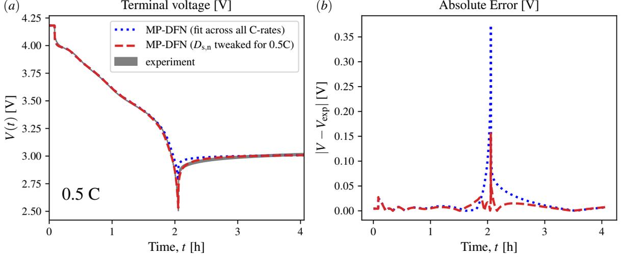
Figure 9: MP-DFN, with parameters fitted across all C-rates, and when  $D_{s,n}$  is then tweaked for 0.5C only. Dotted line is for parameters in Table 2, and dashed line is the same but with  $D_{s,n}$  changed to  $1.30 \times 10^{-13} \text{ m}^2\text{s}^{-1}$ , giving RMSE of 10.3 mV, and cut-off voltage 2.531 V.
