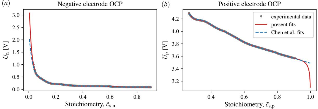
Figure 3: OCP analytical fits to OCP data from [18]. Shown are the fits from Chen et al. [18] (Eqs. 8 and 9 therein), and our fits (Eqs. (34) and (35)) that include logarithmic singularities at  $\tilde{c}_{s,k} = 0, 1$ . (a) Negative electrode  $k = n$  (graphite-SiO<sub>x</sub>); (b) Positive electrode  $k = p$  (NMC 811).
