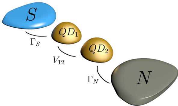
FIG. 1. Schematic view of the quantum dots (QD<sub>1,2</sub>) embedded in series between the normal (N) and superconducting (S) leads with the couplings  $\Gamma_N$  and  $\Gamma_S$ , respectively.
