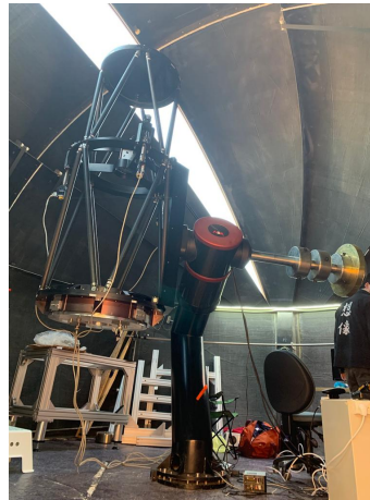
Figure 5. The W-FAST optical tube assembly. Left: CAD image of the mechanical design. Right: the telescope after installation at the observatory.
