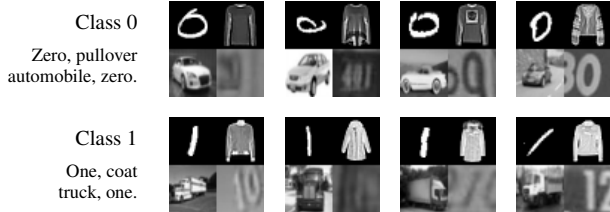
Figure 3. Training examples of collages. Each block features one of two pre-selected classes from MNIST, Fashion-MNIST, CIFAR-10, SVHN. All four blocks are predictive of training labels. Because of the simplicity bias, a standard classifier latches on MNIST and ignores others.
